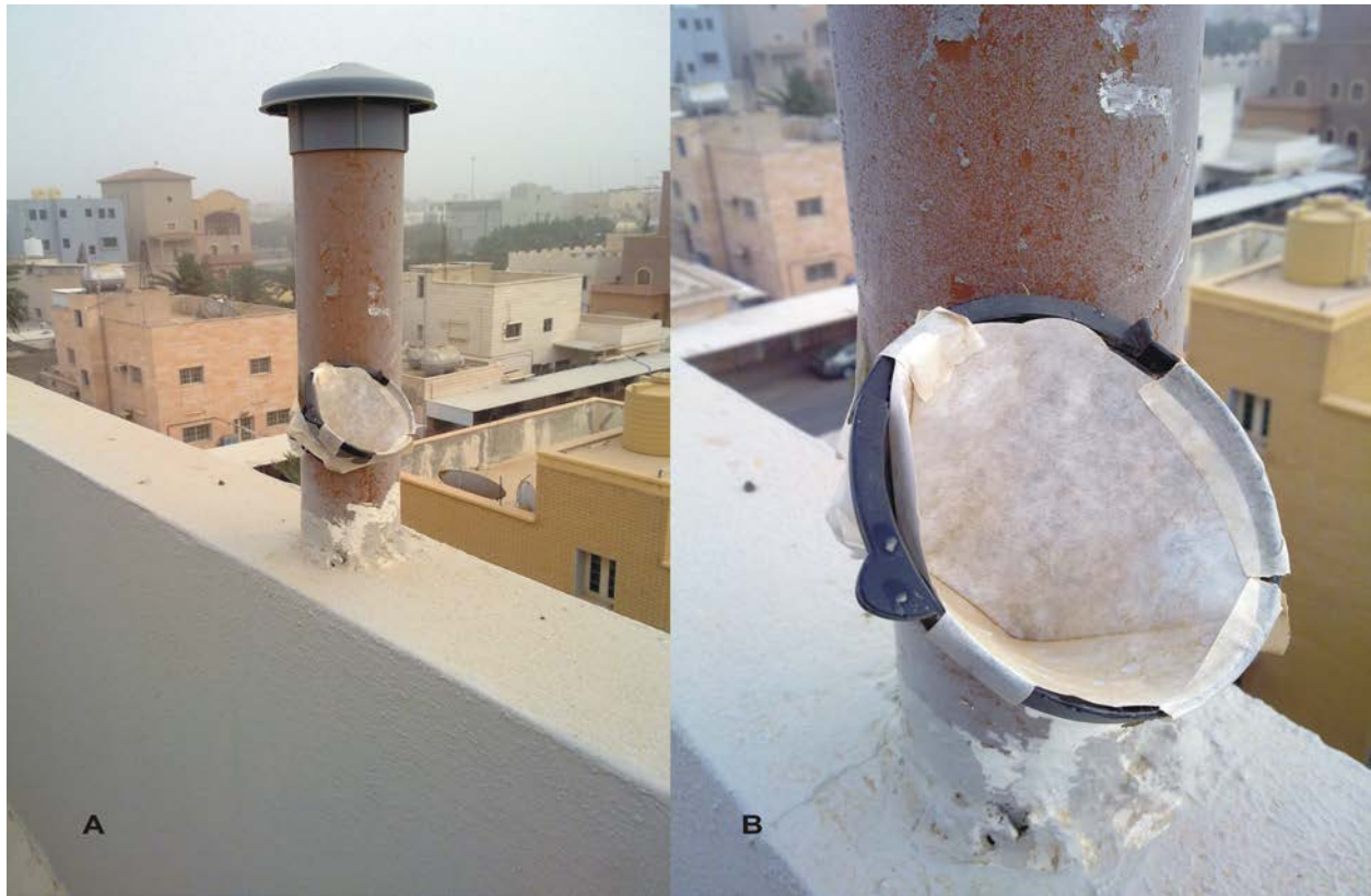
Figure 3.5 A simplified version of the CAPYR method for collecting dust was used. A. General location of the filter, and B. close up of filter, showing a coating of dust.
