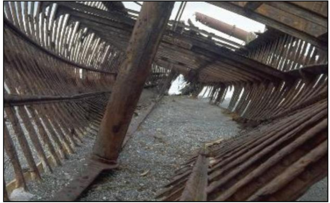
Figure 6.12: A 19 th century composite sailing ship hull structure highlighting the use of I-beams and T-beams. (Histarmar Foundation 2011)
