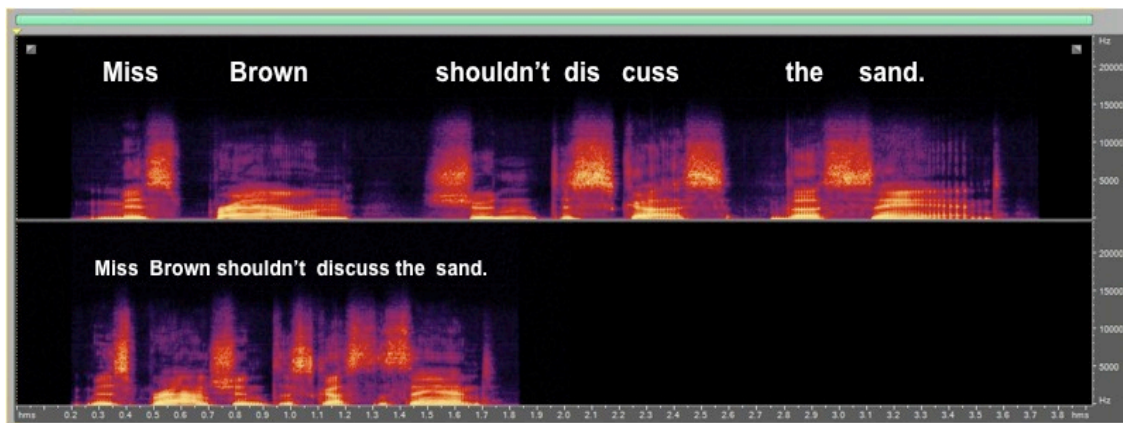
Figure 4-4: Spectrogram demonstrating the vowel duration difference of the word “sand” between clear (top, 379 ms) and conversational speech (bottom, 200 ms)
