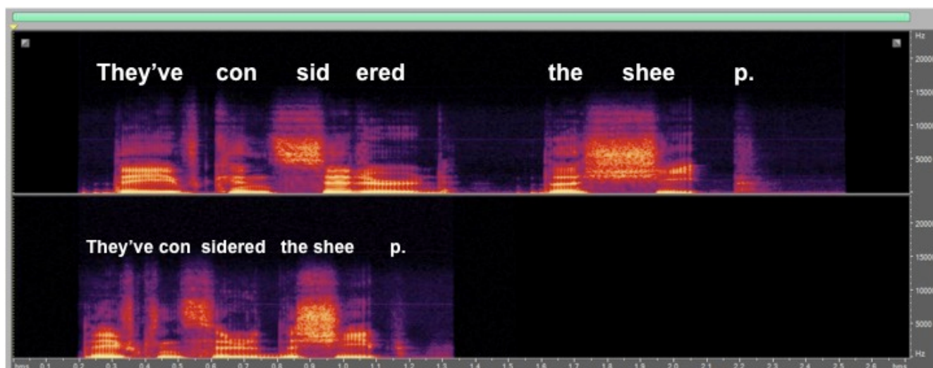
Figure 4-2: Spectrogram demonstrating the intensity and durational differences in the release of the final plosive /p/ of the word “sheep” between clear (top) and conversational speech (bottom).
