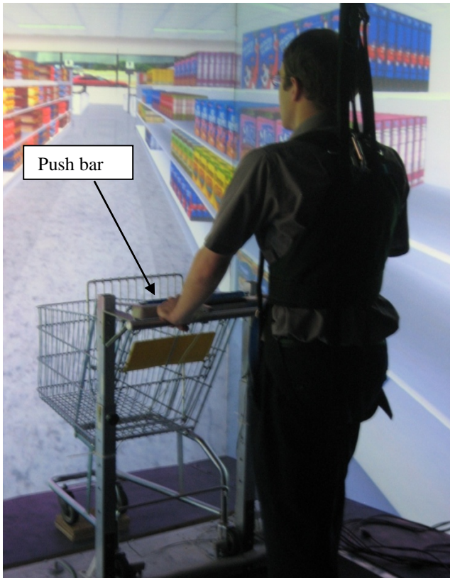
Figure 5-2: The virtual environment is interfaced to a custom-built treadmill with a maximum velocity of 1.2 m/s. A grocery cart at the front end of the treadmill is instrumented with load cells on the push bar to control velocity and movement within the environment
