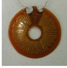
Figure 5.13. A photograph of the annular PZT fiber composite
