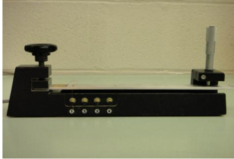
Figure 3.15. The cantilever beam holder and micro-positioning meter for the static strain measurement
