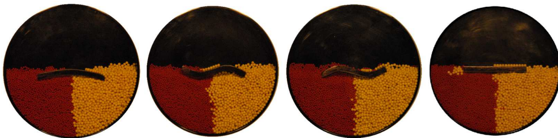
Figure 8: Different baffle shapes considered for this study: C-shaped, S-shaped, Reverse S-shaped and Flat baffle, respectively. Effective length of all types of baffles is constant (equal to the optimum baffle length). The cylinder is rotated at 6 RPM. Also, note that the initial bed is completely segregated with one quarter of the cylinder filled with one kind of particles and the other quarter with the second kind of particles.
