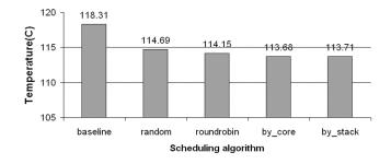
Figure 23: Peak temperatures of different scheduling algorithms.
