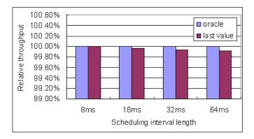
Figure 38: The comparison between the future throughput achieved by using oracle IPC knowledge and the future throughput achieved by using last-value IPC in MBM.
