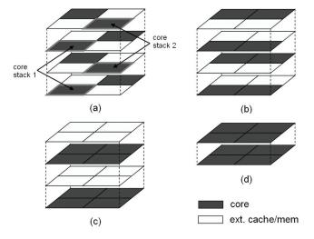
Figure 16: 3D chip multiprocessor floorplan options.
