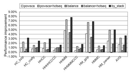
Figure 26: The individual and combined effects of three heuristics. The results are relative to that of the Random scheduler.
