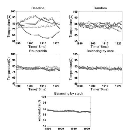
Figure 22: A zoom-in of temperature variation over time under different scheduling algorithms.
