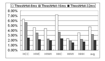
Figure 12: The relative performance improvement by ThreshHot over Baseline, under different scheduling intervals.
