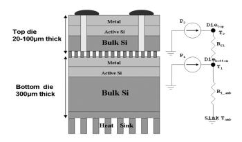
Figure 17: A face-to-back 3D die stacking structure as an example, and the corresponding thermal model.
