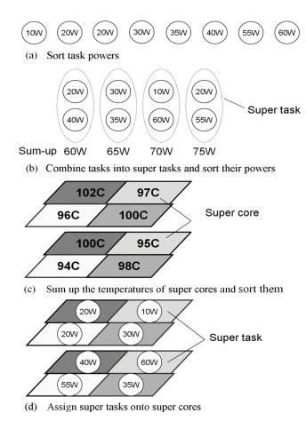
Figure 20: The temperature balancing-by-stack algorithm.
