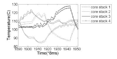
Figure 18: Thermal correlation between adjacent dies.
