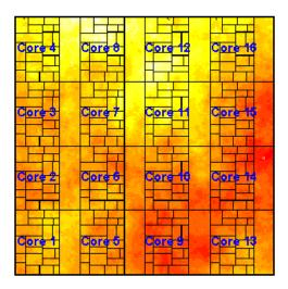
Figure 40: A 16-core CMP with process variation. The colormap under the floorplan shows the within-die variation of the threshold voltage.
