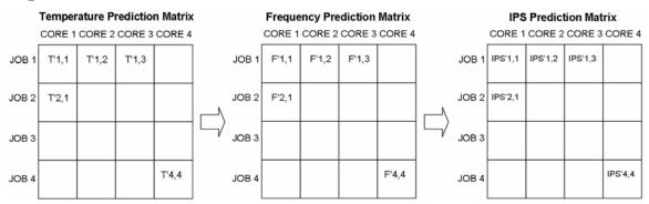
Figure 32: The matrices generated for throughput prediction.
