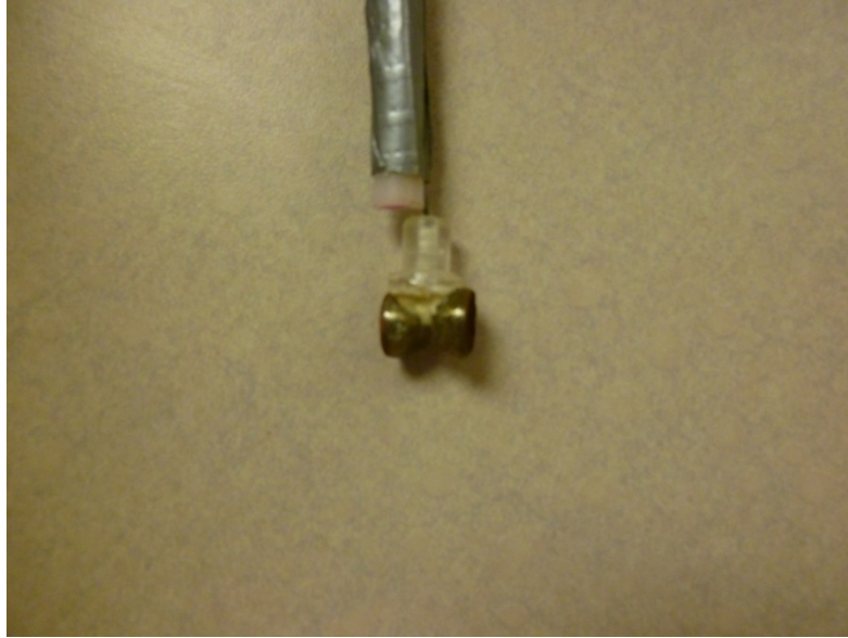
Figure 12. Actual construction of the antenna dipole.
