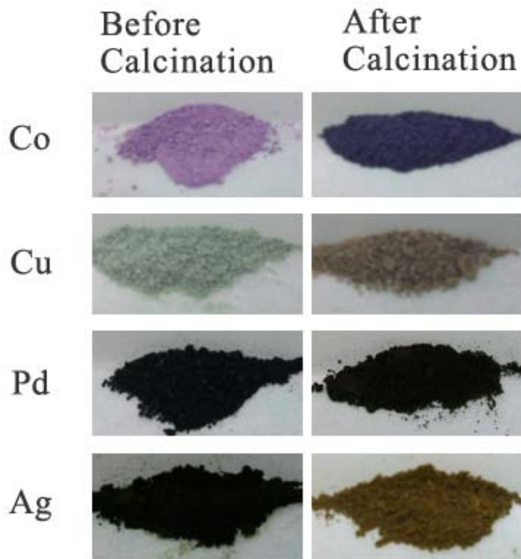
Figure 89: The color of Co@SiO 2 , Cu@SiO 2 , Pd@SiO 2 and Ag@SiO 2 before and after air calcination
