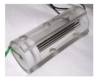
Figure 4.7.1: Image of the linear quadrupole device.
