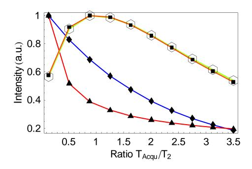
Figure 5.1 Direct, Fourier reconstruction, simulated signal (diamonds), simulated noise (triangles), simulated "experimental" SNR (hollow hexagons). The theoretical formula (boxes) compares excellent with the simulation
