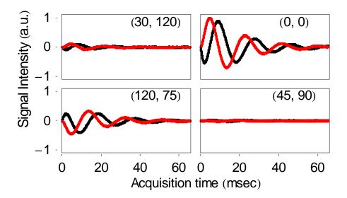
Figure 6.5 the four TQ filtered FID's acquired with different starting phases. Each plot displays the real (black line) and imaginary (red line) parts of the corresponding FID.
