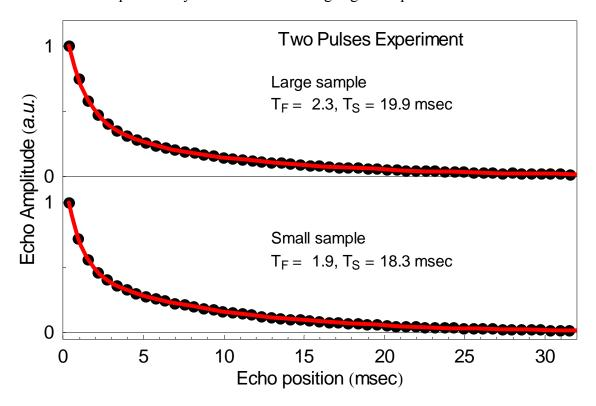
Figure 4.7 Dependence of the NMR signal from a two pulse experiment on the inter-pulse separation for the small agar phantom (lower part) and large phantom (upper part). Each data point corresponds to the peak amplitude of the corresponding FID (TR=209-285ms, 8 averages). The solid line indicates the fit to the signal envelope using the three terms function of the inter-pulse separation t.
