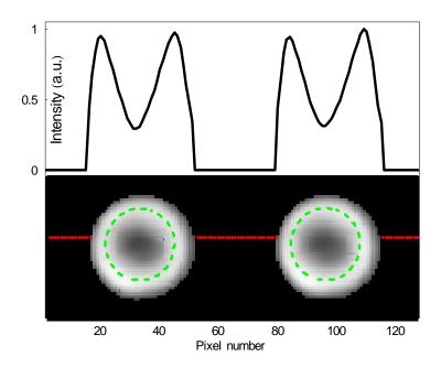
Figure 6.12 The TQ image of the cylindrical phantom. The effect of the off-resonance is visible as a low intensity area, in the center of image
