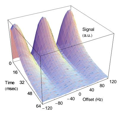
Figure 6.7 the acquired TQ FID magnitudes are displayed as a function of acquisition time and the off-resonance parameter. The vanishing of the TQ signal is expected around  $\delta$ =±50Hz lines and it is well demonstrated by the plot.
