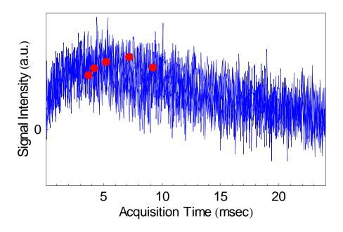
Figure 6.17 Five TQ variable echo experiment using a very inefficient coil. The flip angle was kept far from the 90, in an attempt to reduce the deposited power. The individual FID's are kept hard to visualize, to prove the point that the experimental determination of the optimum preparation time is possible even when the SNR is low. In obtaining the echo amplitudes (dots), the ordering does not change as we change the number involved in averaging between 50 and 100.
