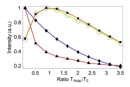
Figure 5.2 Gridding reconstruction, simulated signal (diamonds), simulated noise (triangles), simulated "experimental" SNR (hollow hexagons). The theoretical formula (boxes) compares well with the simulation
