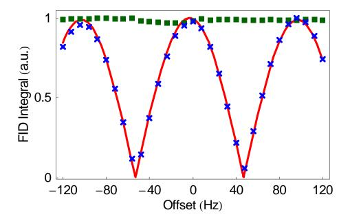
Figure 6.8 integral of the conventional TQ FID as a function of the off resonance parameter (crosses). The theoretical function (solid line) agrees well with experimental data. The modified TQ acquisition data (boxes) shows less variation with the off-resonance parameter.
