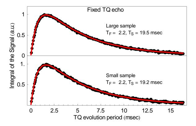
Figure 4.9 Dependence of the integral of NMR signal from a three pulse experiment on the TQ evolution time, for the small agar phantom (lower part) and large agar phantom (upper part). Each data point corresponds to the time integral of the corresponding FID (TR=217-282ms, 10 averages). The solid line indicates the fit to the signal envelope.
