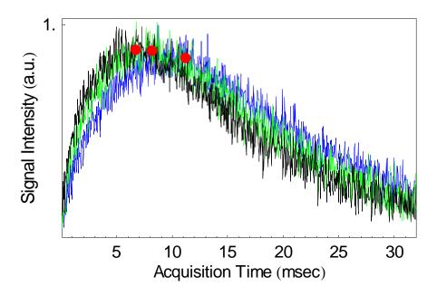
Figure 6.16 Three TQ FID, acquired with the filtering scheme TQ $^-$ , the preparation time is  $\tau_1$ =3.5, 5, and 8 milliseconds. The dots correspond to the echo positions.
