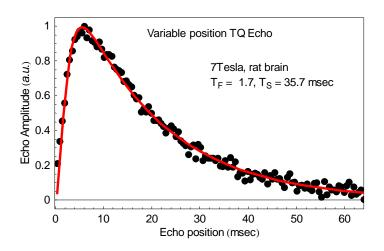
Figure 4.15 Variable echo method applied for a sample consisting of a whole, intact, rat brain. In spite of the low quality of the single FID data, the 2D acquisition is able to retrieve correct physical quantities.
