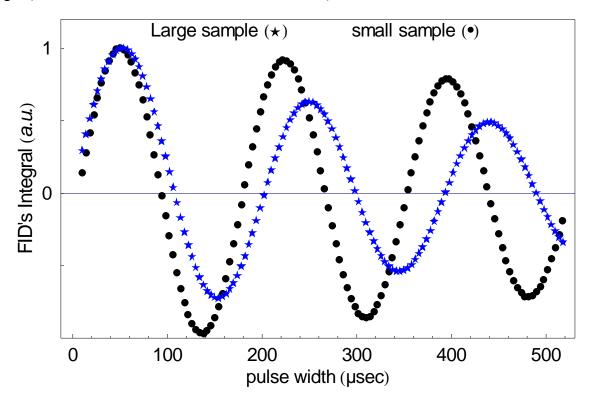
Figure 4.6 Dependence of the NMR signal on the RF pulse length for the small (bullets) and the large (stars) samples. Each data point corresponds to the integral of the FID (TR=191ms, 16 averages) following the RF pulse with corresponding pulse width.
