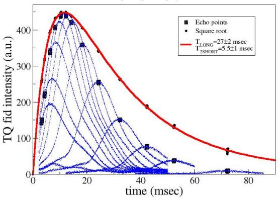
Figure 6.9 Variable echo experiment, the sample used, described in the text, is characterized by large  $B_0$  inhomogeneities, therefore the indivifual FID's are distorted from the biexponential form. Selecting only the echo amplitudes and representing their square root values (bullets) the biexponential form is obtained with the  $T_{\rm LONG}$  of 27 milliseconds and  $T_{\rm SHORT}$  5.5 milliseconds.
