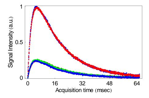
Figure 6.6 the four individual components (the overlapping, low amplitude FID's) are displayed together with the reconstructed and on-resonance signals (the overlapping, high amplitude FID's).
