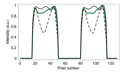
Figure 6.15 The conventional TQ profile (dashing) and modified TQ (thick solid line), together with the SQ profile (thin solid line). The variation in the reconstructed intensity observed in the corrected TQ image is due to the presence of  $B_1$  inhomogeneity, ringing and intravoxel dephasing. However, a significant source of variation has been removed by using modified TQ scheme
