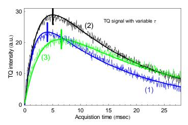
Figure 4.12 TQ FID's acquired on a small agar sample, using the Signa GE scanner and a solenoid coil. The FID's correspond to preparation times of 3, 5 and 8 milliseconds. As expected, the position of the maximum TQ signal depends on the preparation time, a clear sign of  $B_0$  inhomogeneities across the sample. The solid lines represent biexponential fit of each data.
