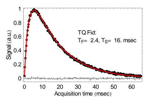
Figure 6.2 The conventional TQ filtered FID. The fit to a biexponential function (solid line) is presented together with the experimental real (dots) and imaginary (thin line) data points. The displayed data points are undersampled, to simplify the graph.
