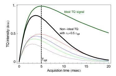
Figure 4.11 Behavior of non-ideal TQ with the variation of the preparation time. Thin lines represent the four components, while the thick dark line is their sum (scaled to half of its value, for display purposes)
