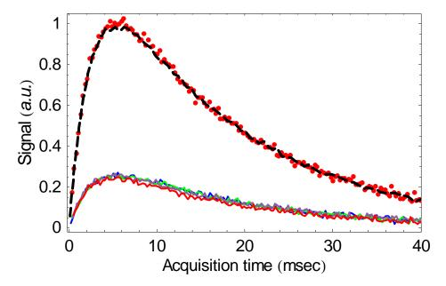
Figure 6.3 The on-resonance conventional TQ signal (dashed line) compared with signals originating from individual coherence pathways (solid lines) and their sum (dots).
