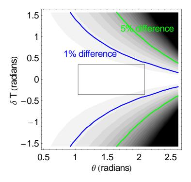
Figure 2.2 The contour plot of the difference between the exact expression  $T_{\theta,\delta}$  and the approximate  $T_{\theta}$
