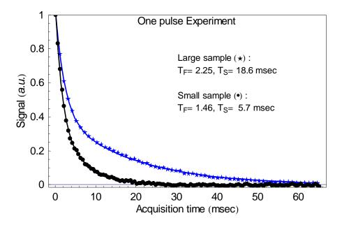
Figure 4.5 FID and non-linear fit using the biexponential, from a one pulse experiment on the small agar phantom (bullets) and the large agar phantom (stars). (TR=191ms, 8 averages).
