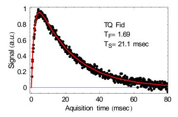
Figure 4.16 TQ FID obtained on a sample consisting of five intact mice brains. Due to the fact that the sample is placed in saline solution, the  $B_0$  homogeneity is improved. Still, the values obtained by fitting are biased.
