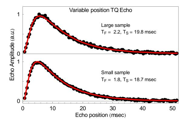
Figure 4.8 Dependence of the NMR signal from a three pulse experiment on position of the echo (a function of the inter-pulse delay) for the small (lower part of the plot) and large (upper part of the plot) agar phantom. Each data point corresponds to the amplitude of the echo (TR=157-259ms, 20 averages). The solid line indicates the fit to the signal envelope, as described in text.
