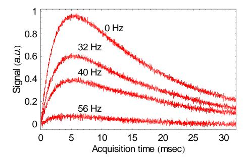
Figure 6.4 the conventional TQ signal for four different settings of the off-resonance parameters (0, 32, 40, and 56 Hz). Each signal is phase corrected to 0<sup>th</sup> and 1<sup>st</sup> orders. As expected, the TQ intensity is significantly diminished as the off-resonance increases.
