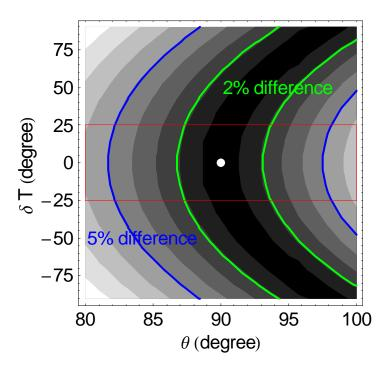
Figure 2.3 The difference between the effective length of a 90 degree pulse and a  $\theta$  pulse, as a function of inhomogeneity and flip angle.
