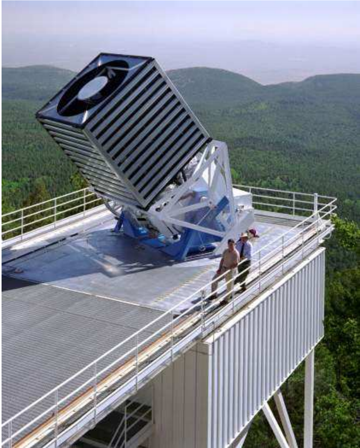
Figure 3.1: The SDSS 2.5m telescope at Apache Point Observatory. Credit: Fermilab Visual Media Services.
