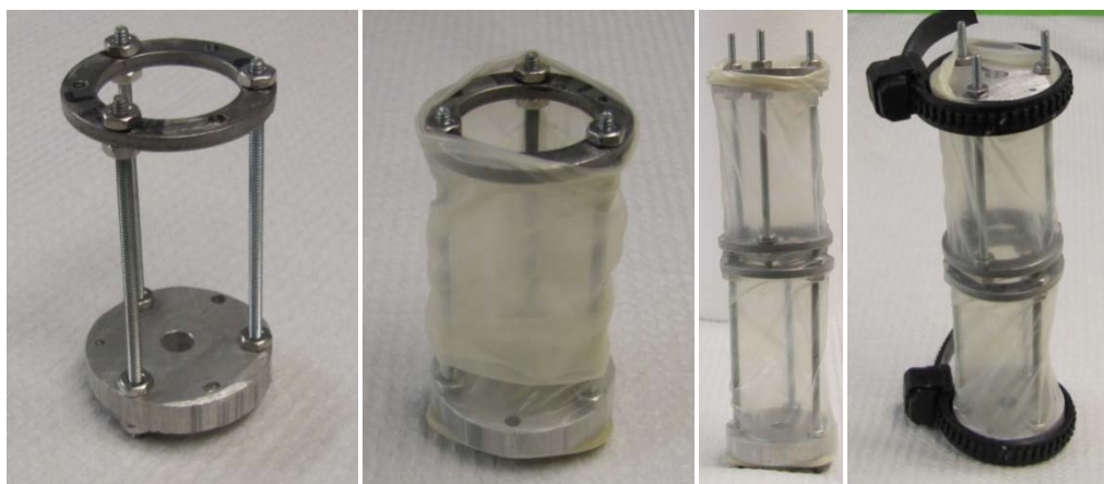
Figure 3. Ring-and-post design with flexible-walled membrane
