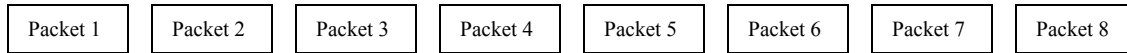
Figure 5.5: A diagram of eight separate packets of 8 bits each totaling 64 bits from a single tag
