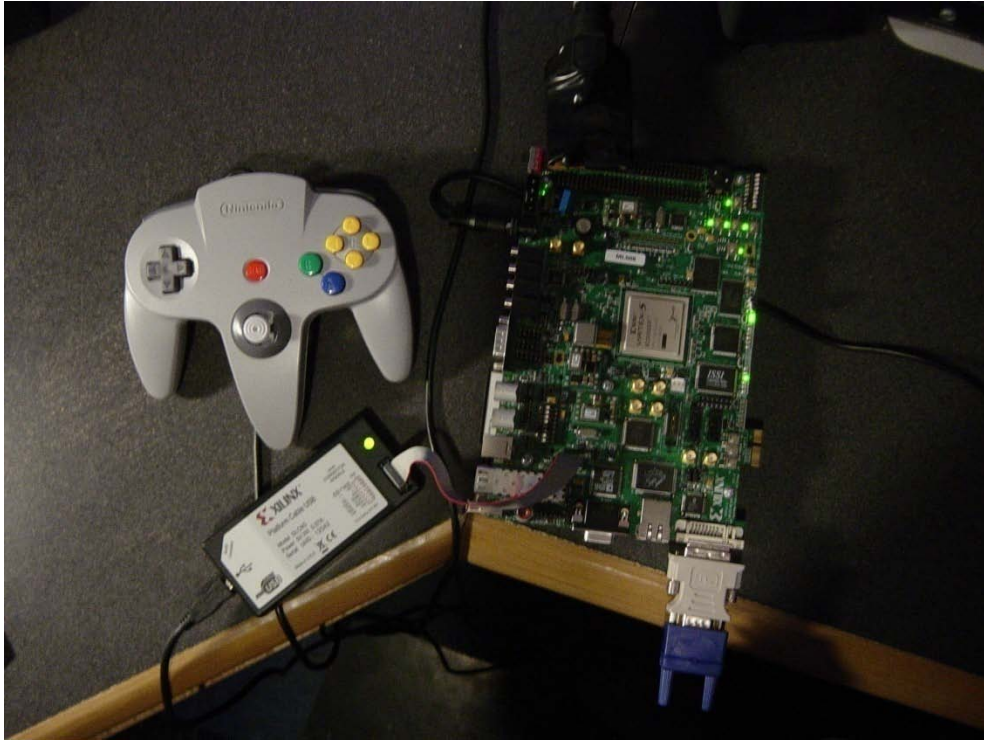
Figure 4.45: Development Kit with JTAG, VGA and N64 Hardware
