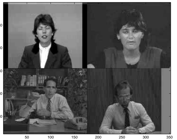
(g) DCT-SPIHT, 15000 bits PSNR=34.4821 dB
