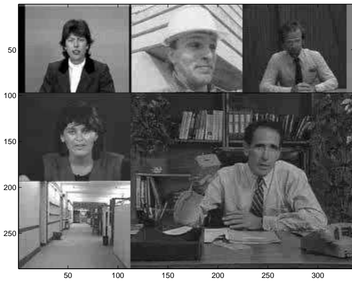
(f) Conventional DCT (QP=10), 33959 bits PSNR=32.1421 dB
