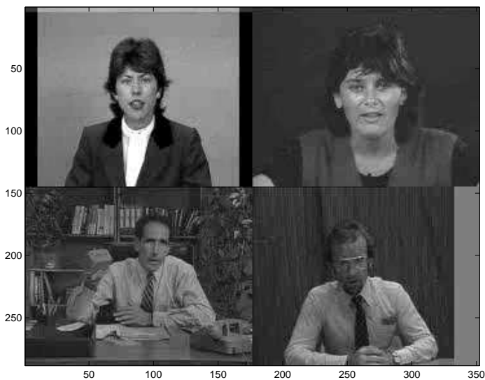
(f) Conventional DCT (QP=10), 30042 bits PSNR=33.4238 dB
