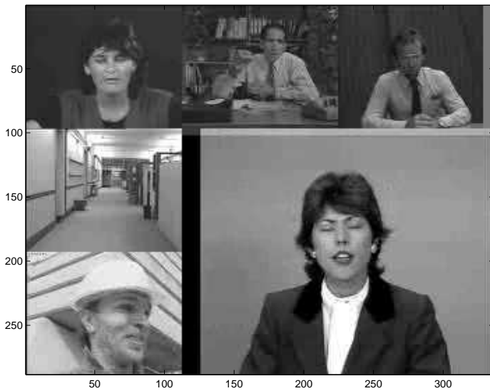
(f) DCT-EZT, 15000 bits PSNR=32.4553 dB
