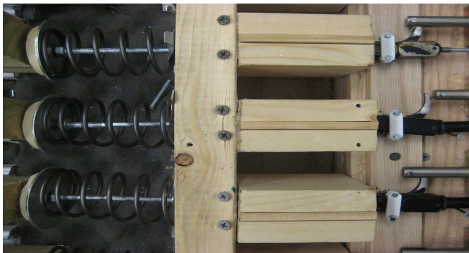
Figure 5. Complete trigger assembly: solenoid, trigger, eyebolt, spring, slide.
