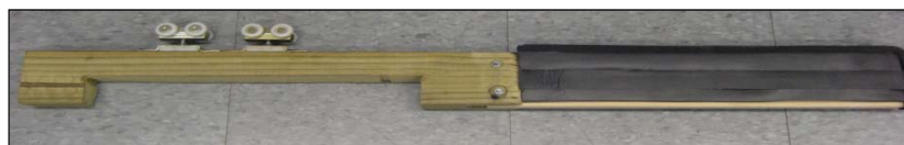
Figure A.B.2. Wood tripper slide with padding.
