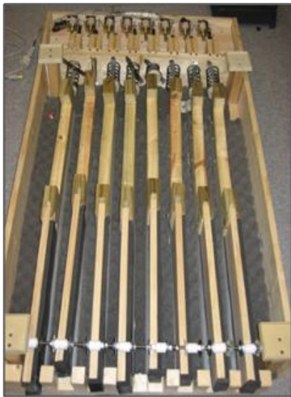
Figure 4.1 Tripping device (bottom side up (left) and solenoid-caliper-eyebolt-spring assembly (right).
