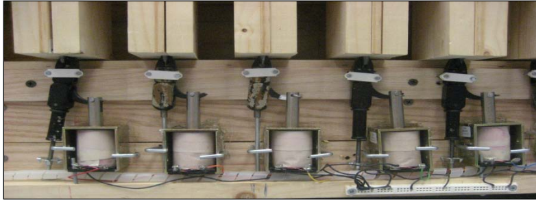
Figure A.B.3. Solenoid and trigger with eyebolt locked in trigger head.
