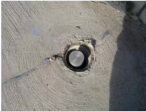
Figure 5.3 Top of invar rod.
