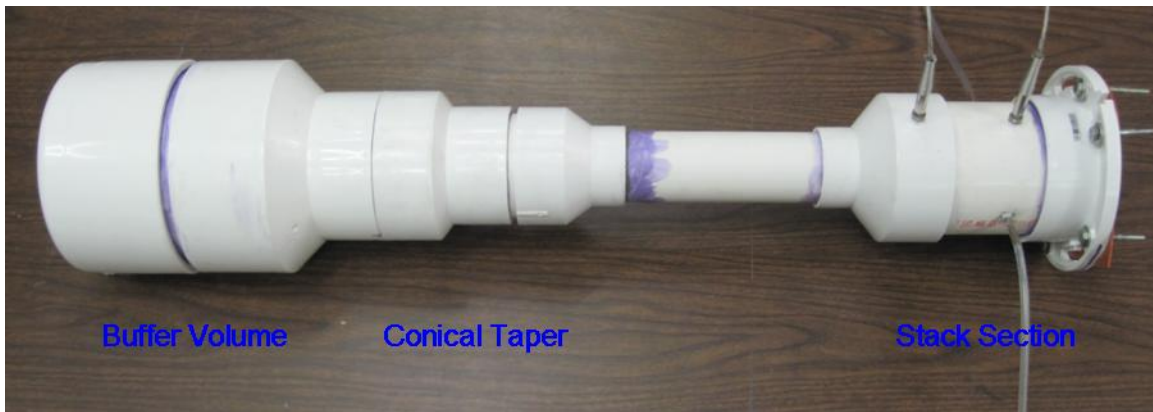
Figure 13. Resonator with two thermocouples, stack, and heat exchanger installed.
