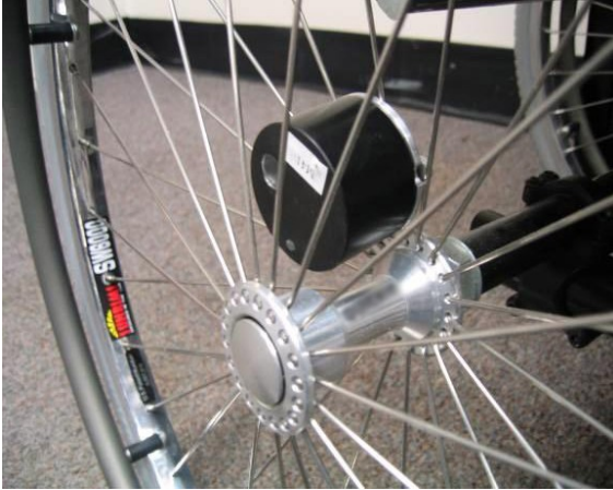
Figure 6. Shows the data logger mounted to the spoke of a manual wheelchair.
