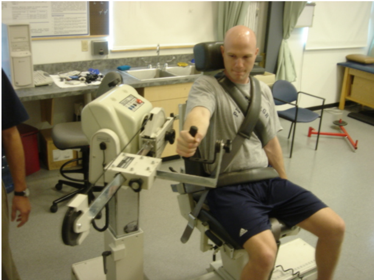
Figure 8 Biodex setup for shoulder protraction/retraction strength assessment
