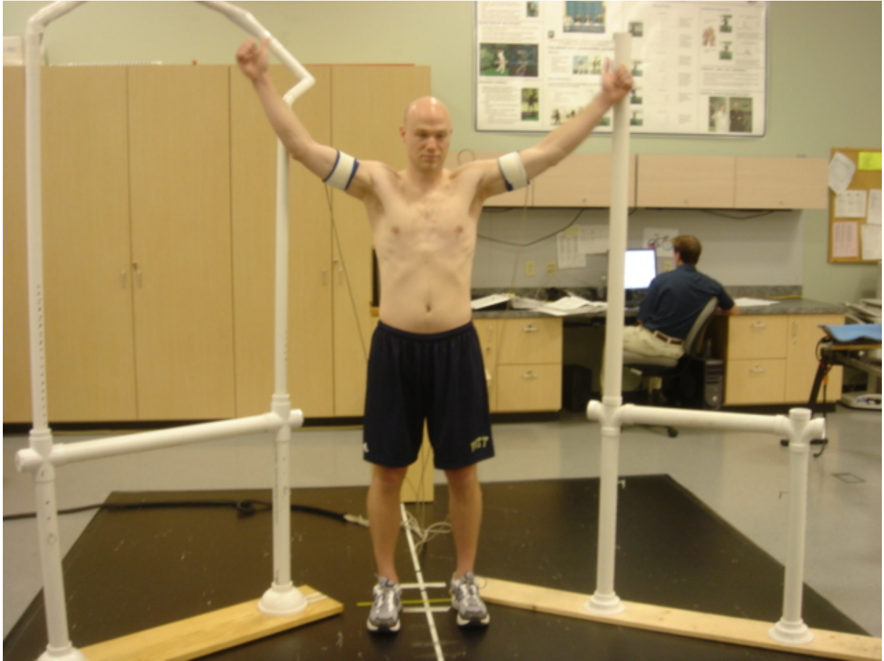
Figure 6 Plastic guide tubes to keep elevation in scapular plane
