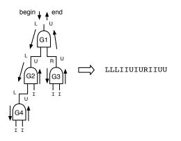
Figure 3: A simple circuit to illustrate the generation of LURU string representations.
