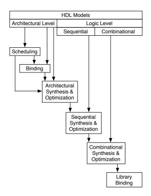
Figure 1: A synthesis and optimization design flow for digital integrated circuits according to De Micheli [1].
