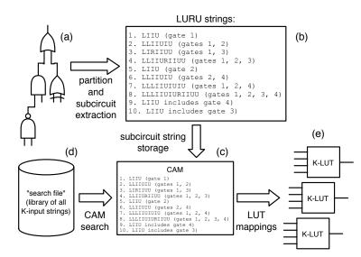
Figure 2: FPGA technology mapping design flow using LURU with CAM.
