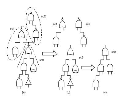
Figure 5: The input circuit in (a) is partitioned into subcircuits sc1, sc2, and sc3 in (b) at the point of multiple fanout. Subcircuit sc3 is represented in (c) without the inverter and with generic gate types, as permitted by property P1 in Section 3.1.
