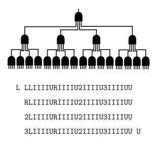
Figure 7: Homogeneous LURU circuit topology expressed as an HLS (homogeneous LURU string).
