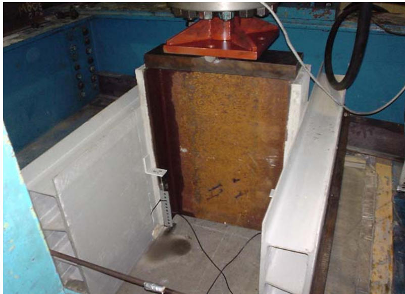
Figure 1-4: Push-off Test Specimen in Load Frame (Yulisman 2005)
