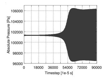
Figure 59: First replication of thermoacoustic oscillations, transitioning from amplification to approaching a steady state (called the limit cycle by Hanschke et al.)
