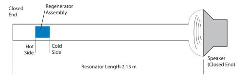
Figure 27: Schematic view of the TAR setup
