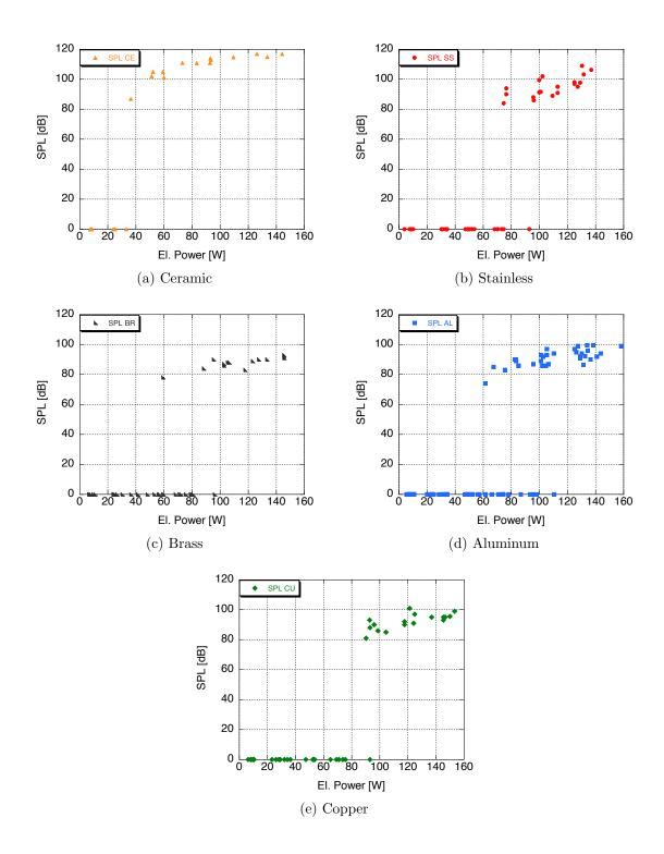
Figure 117: Sound pressure level achieved by each stack as a function of input power, ranging from materials with low thermal conductivity (a) to high thermal conductivity (e)
