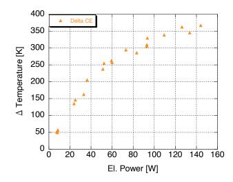
Figure 20: Temperature difference across the ceramic stack.
