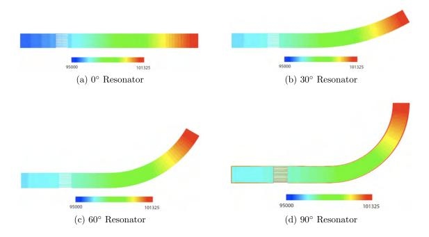
Figure 89: Pressure distribution for the whole domain for four cases of resonator curvature.
