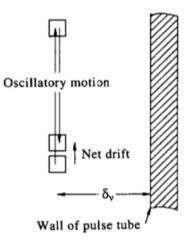
Figure 8: Illustration of drift (Gedeon streaming) resulting from variations in viscosity in the working gas in a pulse tube refrigerator
