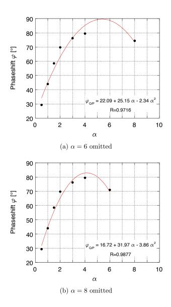
Figure 103: Phase difference between pressure and heat transfer and quadratic curve fits, omitting either  $\alpha = 6$  or  $\alpha = 8$ .
