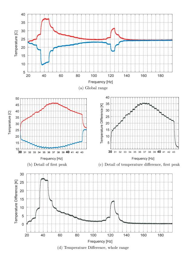
Figure 31: Illustration of the temperature difference across the regenerator as a function of driving frequency.
