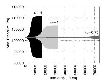
Figure 104: Illustration of the approaching stability limit, where an amplification of the pressure amplitude does not occur,  $\alpha = 4$ ,  $\alpha = 1$  and  $\alpha = 0.75$  shown.
