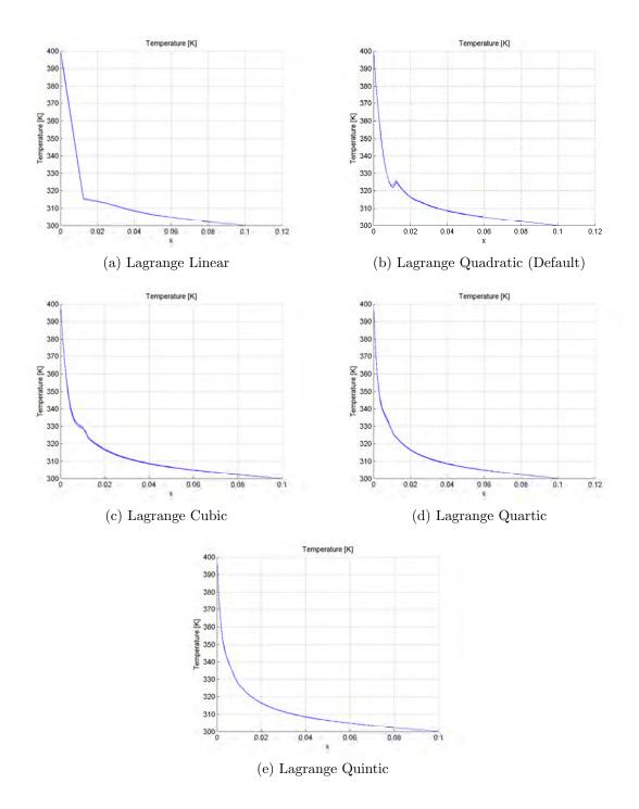
Figure 120: Illustration of the surface temperature distribution for a fixed domain size as a function of element type (Linear through quintic). Higher order elements minimize errors.
