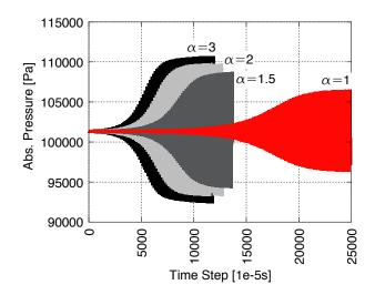
Figure 94: Pressure behavior for four values of  $\alpha$  (1, 1.5, 2, and 3), compared to the physical case.
