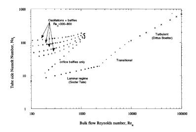
Figure 55: Heat transfer behavior of tube flow subject to oscillations, compared to laminar, transitional, and turbulent heat transfer correlations.
