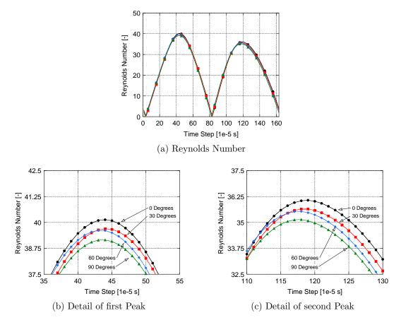
Figure 74: Comparison of the Reynolds number behavior under the influence of different degrees of resonator curvature.
