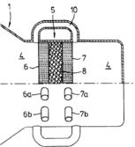
(b) Thermoacoustic device with a feedback inertance (Position 10), one of four suggested designs introduced by deBlok et al.
