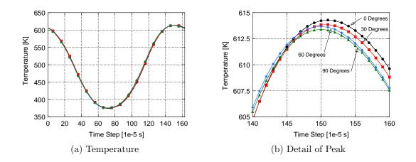
Figure 76: Comparison of temperature behavior under the influence of different degrees of resonator curvature.
