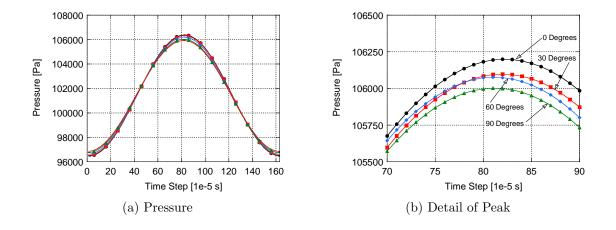
Figure 70: Comparison of pressure behavior under the influence of different degrees of resonator curvature.
