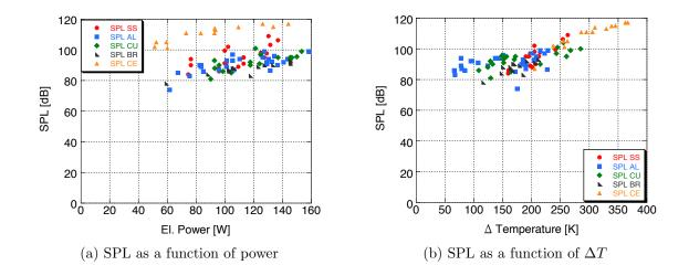
Figure 21: Illustration of the achieved sound pressure level as a function of electrical input power and temperature difference  $\Delta T$
