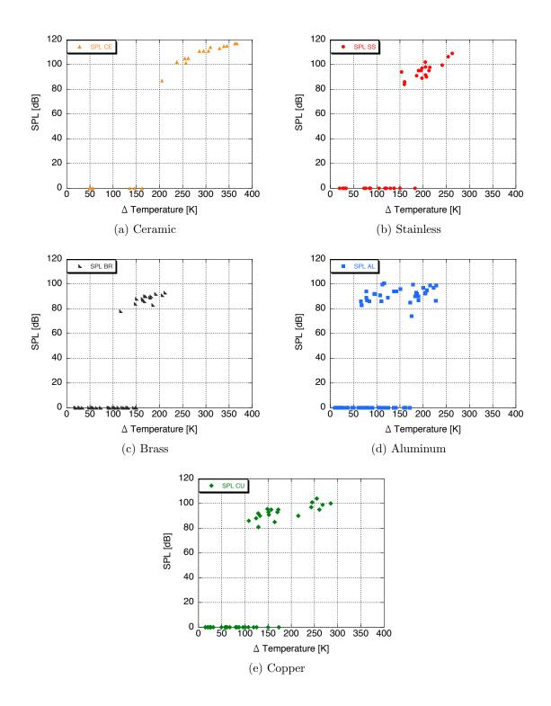
Figure 116: Sound pressure level achieved by each stack as a function of temperature difference, ranging from materials with low thermal conductivity (a) to high thermal conductivity (e)
