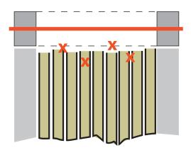
Figure 17: Placement of thermocouples near the hot side heat exchanger as a source of inconsistent measurements
