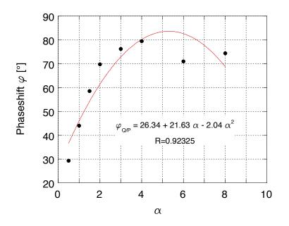
Figure 102: Phase difference between pressure and heat transfer as the thermal conductivity of the gas is increased.
