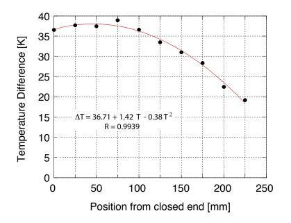
Figure 32: Temperature difference as a function of regenerator location relative to the closed end (measurement locations are spaced  $25 \ mm$  apart)
