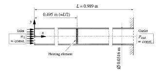
Figure 48: Rijke tube as modeled by Hanschk et al.
