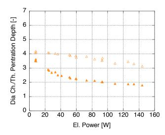
Figure 24: Ratio of channel size and thermal penetration as a function of input power (solid symbols: hot side, outlined symbols: cold side), for the ceramic stack.
