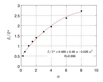
Figure 99: Change in thermal penetration depth as the thermal conductivity is increased.
