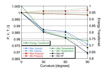
Figure 93: Illustration of the dependence of pressure, velocity, temperature, heat transfer and energy transfer on resonator curvature (normalized).
