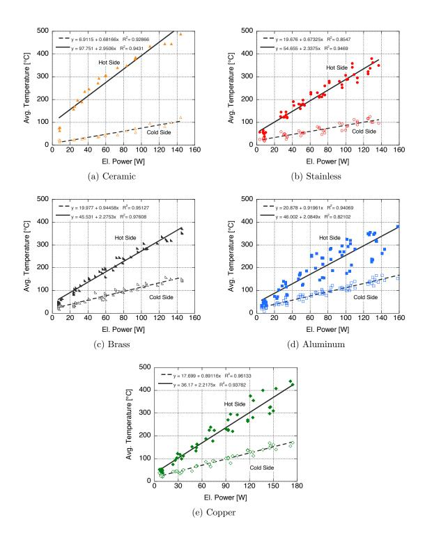
Figure 114: Hot side and cold side temperature, including linear curve fits, for various stack materials ranging from low thermal conductivity (a) to high thermal conductivity (e)
