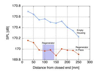
Figure 30: Illustration of the SPL achieved in the regenerator housing empty, and with the regenerator assembly in place.
