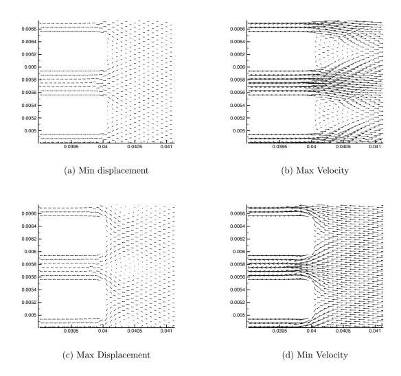
Figure 85: Velocity vectors at the cold side
