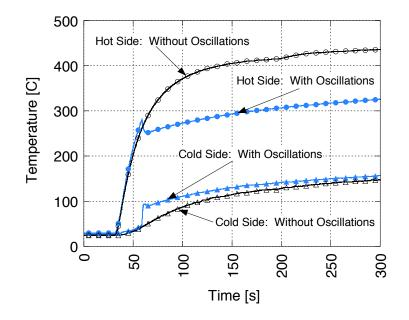
Figure 12: Temperatures on both ends of the stack in a standing wave engine. The heating of the ambient side is apparent
