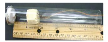
Figure 4: Simple standing wave engine demonstrator, built with Pyrex tubing, and a 600cpi ceramic monolith stack.
