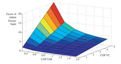
Figure 7: Illustration of the additional energy required to drive a thermoacoustic refrigeration system when it replaces a vapor compression refrigeration system
