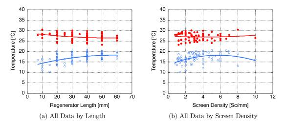
Figure 43: Plots showing all data for  $100\mu m$  stainless steel, whole range of number of screens and regenerator length
