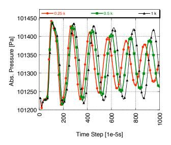
Figure 97: Pressure behavior for three different Prandtl numbers (physical,  $\times 2$ , and  $\times 4$ ) by variation of the thermal conductivity.
