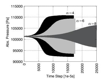
Figure 95: Pressure behavior for three values of  $\alpha$  (4,6, and 8), compared to the physical case.
