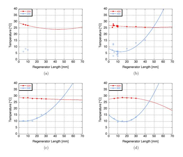
Figure 38:  $105\mu m$  Nylon, temperature data separated by screen count, as a function of regenerator length, part 1: 20-60 screens
