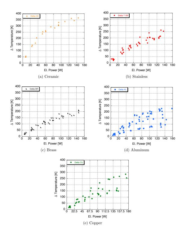
Figure 115: Temperature difference across the stack ranging from materials with low thermal conductivity (a) to high thermal conductivity (e)
