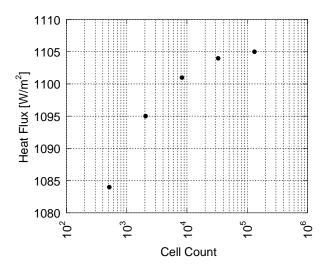
Figure 110: Illustration of the error resulting from using a coarse mesh rather than a refined mesh in COMSOL. The error is less than 2% and not expected to rise further with increasing cell count.
