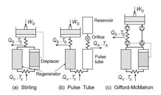
Figure 6: Illustration of three main thermoacoustic refrigerator types
