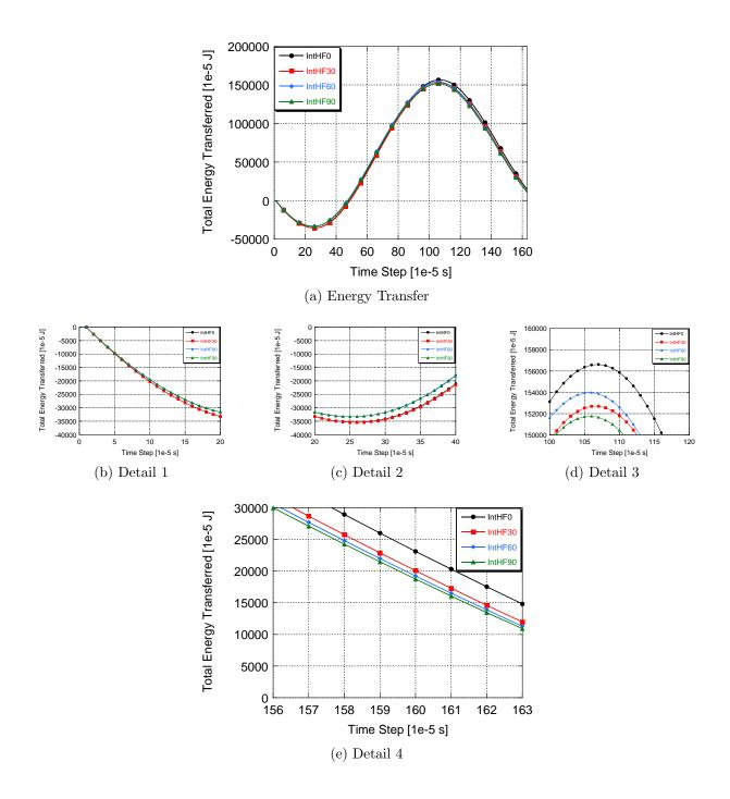
Figure 78: Energy transferred ( $\Delta E$ ) for the horizontal stack surface. Comparing four different resonator shapes (0°, 30°, 60°, 90°).
