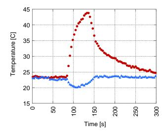
Figure 11: Illustration of heat driven refrigeration: Cooling at onset of oscillation (80 seconds) and subsequent heating of the cold side because of addition of heat from driving stack via unchecked streaming
