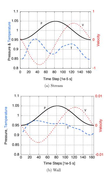
Figure 67: Comparison between free stream and wall temperature, pressure, and velocity behavior at the hot end of the stack revealing the influence of pressure on the temperature change.
