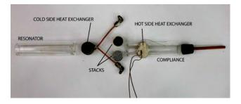
Figure 15: Exploded view of the engine components: resonator, cold side heat exchanger, stacks, hot side heat exchanger, and compliance
