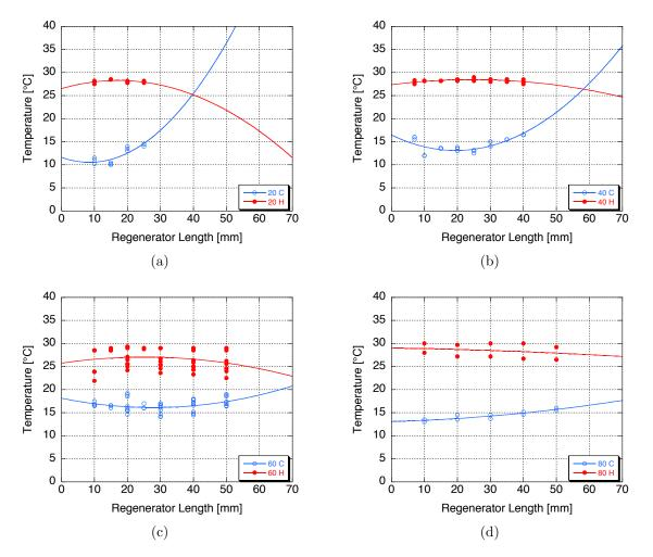
Figure 44:  $100\mu m$  stainless steel, temperature data separated by screen count, as a function of regenerator length, part 1: 20-80 screens.
