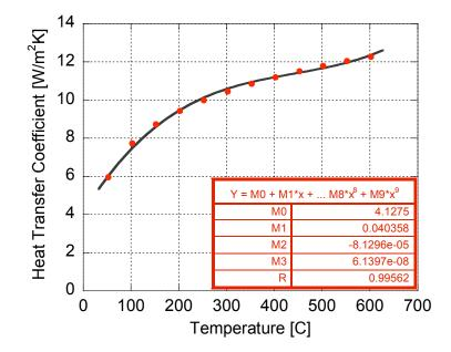
Figure 25: The heat transfer coefficient and its curve fit over the relevant range of temperatures
