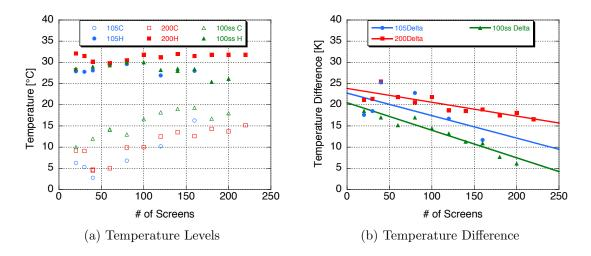
Figure 46: Plots showing the temperature levels (maximum  $T_{hot}$  and minimum  $T_{cold}$ ) for each material and screen count.
