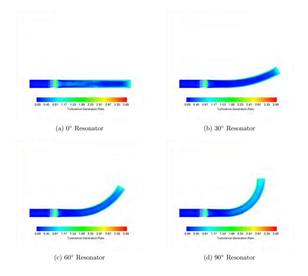
Figure 91: Turbulence generation for the whole domain for four cases of resonator curvature.
