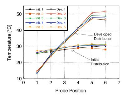
Figure 35: Direct comparison between each case and measurement location, for two different times: initial distribution and an established case (after  $\approx 10$  minutes).
