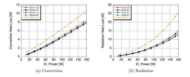
Figure 26: Estimates of the convective and radiative heat flux around the stack assembly
