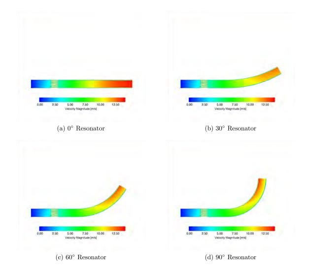
Figure 90: Velocity field for the entire domain for four cases of resonator curvature.
