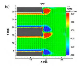
Figure 87: Vortex structure at the stack outlet, as measured through PIV by Mao et al.
