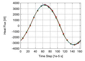
Figure 77: The integrated heat flux ( $Q_{int}$ , as derived in Equation 6.7) over the horizontal stack surfaces, comparing four different resonator shapes ( $0^{\circ}$ ,  $30^{\circ}$ ,  $60^{\circ}$ ,  $90^{\circ}$ ).
