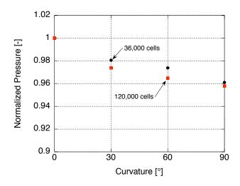
Figure 61: Illustration of the difference in pressure amplitude between the various curved resonator geometries.
