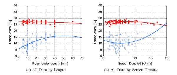
Figure 37: Plots showing all data for  $105\mu m$  Nylon, for the whole range of the number of screens and regenerator length
