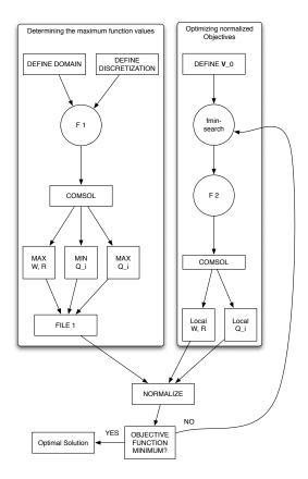
Figure 109: Flow diagram of the optimization routine, including the preprocessor
