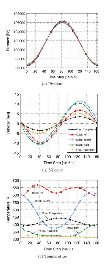
Figure 65: Pressure, velocity, and temperature measured in the center/stream location, straight resonator.
