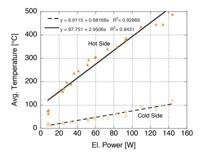
Figure 18: Hot side and cold side temperature across the ceramic stack.
