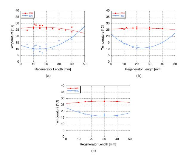
Figure 39:  $105\mu m$  Nylon, temperature data separated by screen count, as a function of regenerator length, part 2: 80-160 screens
