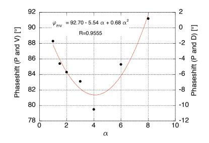
Figure 101: Change in phase shift between pressure and velocity as the thermal conductivity of the gas is increased.
