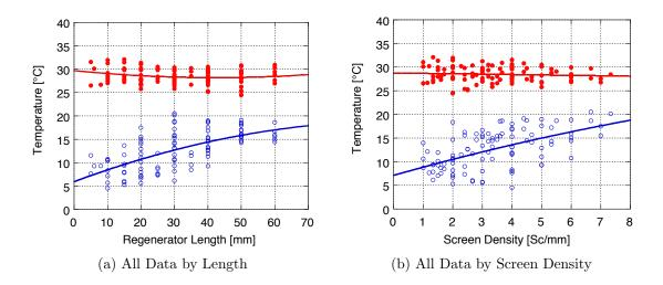
Figure 40: Plots showing all data for  $200\mu m$  Nylon, for the whole range of number of screens and regenerator length
