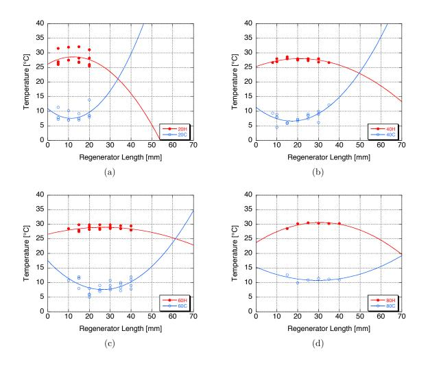
Figure 41:  $200\mu m$  Nylon, temperature data separated by screen count, as a function of regenerator length, part 1: 20-80 screens.
