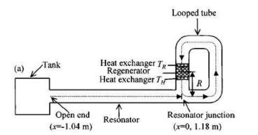
(a) Thermoacoustic engine with looped feedback path, by Ueda et al.
