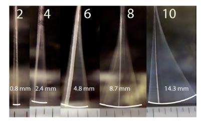
Figure 47: Illustration of the displacement throughout the regenerator housing: measurement position 2 is located at 50 mm, and each subsequent position an additional 50 mm further away.
