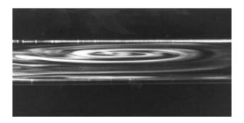
Figure 10: Vortex formed by streaming inside the resonator of a thermoacoustic engine
