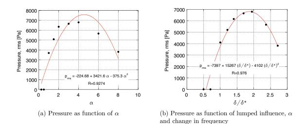
Figure 100: Change in pressure amplitude as the thermal conductivity is increased, shown as a function of  $\alpha$  directly and as a function of (normalized) thermal penetration depth.
