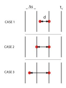
Figure 36: Three ratios of displacement to screen spacing: Case 1 is  $d/\delta s < 1$ , Case 2  $d/\delta s = 1$ , Case 3  $d/\delta s > 1$ .
