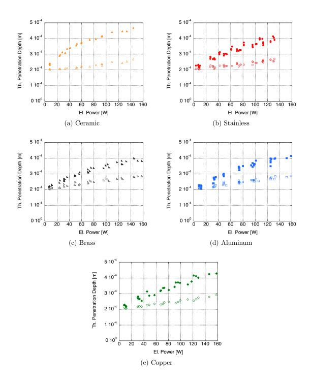
Figure 118: Thermal penetration depth as a function of input power for each stack material, ranging from materials with low thermal conductivity (a) to high thermal conductivity (e)
