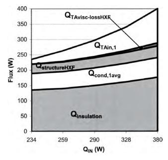
Figure 13: Energy balance of a thermoacoustic engine as a function of heat input
