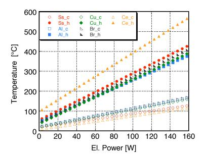
Figure 19: Curve fits of the temperature behaviors depending on stack material
