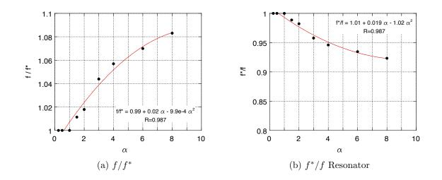
Figure 98: Change in operating frequency (normalized with respect to physical case) and its inverse (as used in Equation 7.3) as the thermal conductivity is increased.
