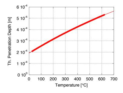
Figure 22: Thermal penetration depth  $\delta_{\kappa}$  as a function of temperature
