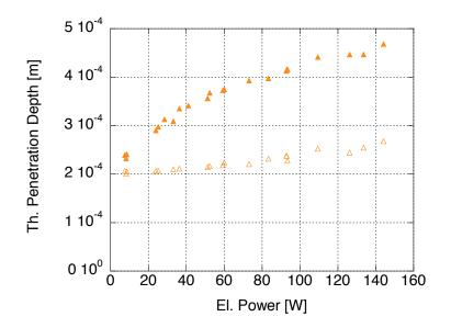
Figure 23: Thermal penetration depth as a function of input power (solid symbols: hot side, outlined symbols: cold side) for the ceramic stack.
