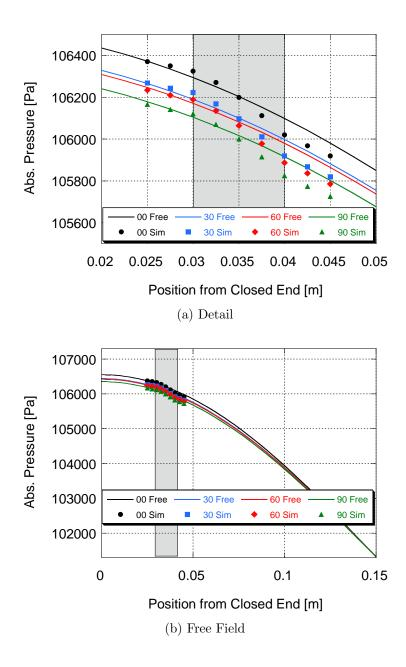
Figure 92: Pressure peaks throughout the stack, and comparison with the free field pressure distribution of a standing wave.
