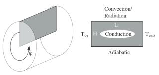
Figure 106: Illustration of computational domain and implemented boundary conditions
