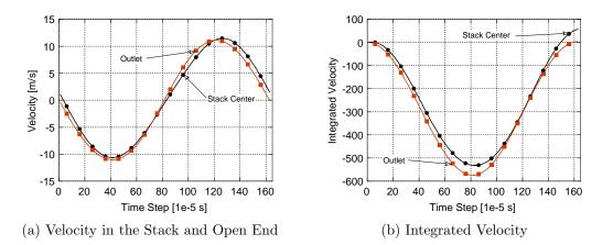
Figure 72: Comparison of velocity behavior in the stack and the outlet for the straight resonator (velocity antinode).
