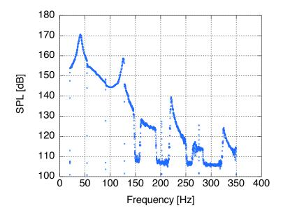
Figure 29: Sound pressure level as a function of driving frequency.
