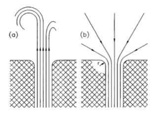
Figure 9: Illustration of flow behavior of a gas flowing leaving a small (a) tube as opposed to entering it (b)
