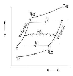
Figure 2: T-s Diagram for Stirling Cycle
