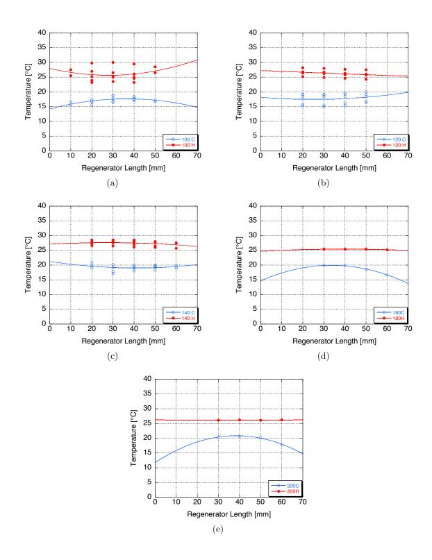
Figure 45:  $100\mu m$  stainless steel, temperature data separated by screen count, as a function of regenerator length, part 2: 100-200 screens
