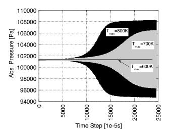
Figure 62: Sensitivity of the solution to the prescribed temperature profile, hot side temperatures of 800 K, 700 K, and 600 K. The cold side is constant at 300 K
