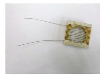
Figure 14: Hot side heat exchanger, ceramic frame with NiCr wire woven through it
