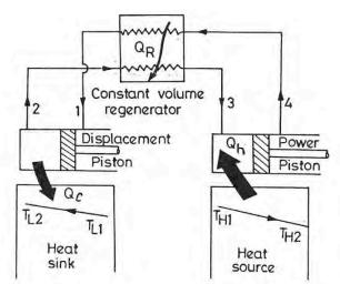
Figure 1: Schematic of Stirling Engine
