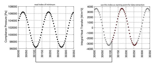
Figure 69: Illustration of the collection of data relative to the minimum of the compliance pressure (after 30000 timesteps)
