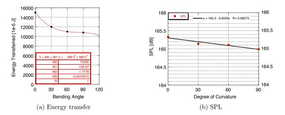
Figure 79: Effect of the curvature on energy transfer and sound pressure level
