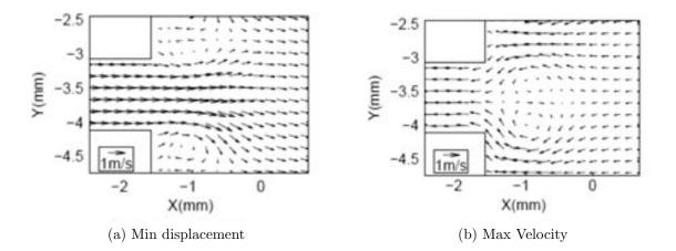
Figure 86: Velocity vectors as a result from PIV investigation of the thermoacoustic effect as published by Berson et al.
