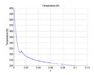
Figure 107: Error in the temperature distribution resulting from use of quadratic mesh elements
