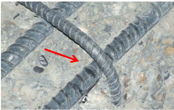
(a) location of bar fracture (beam is inverted, cover has been removed).
