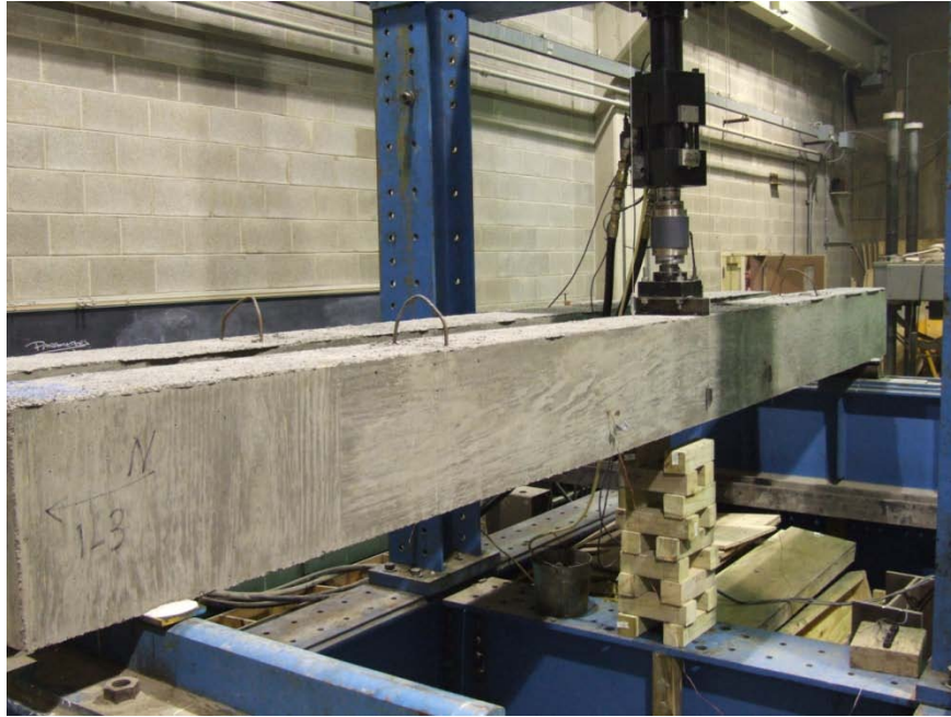
(a) Fatigue specimen test 1, before loading
