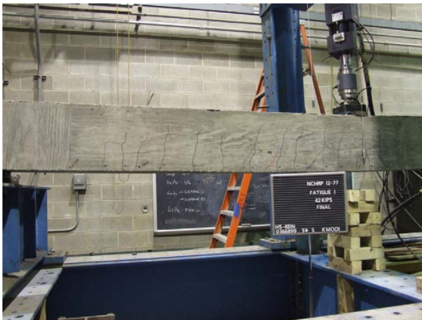
(b) Fatigue specimen test 1 at 2 million cycles
