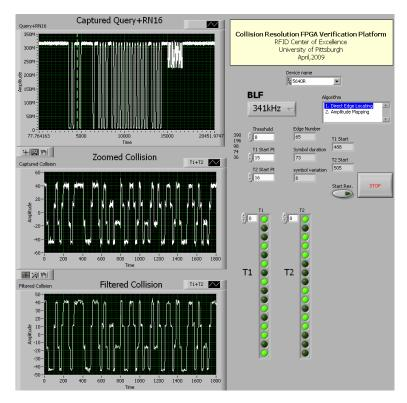
Figure 53. Resolution Result When BLF=341 kHz
