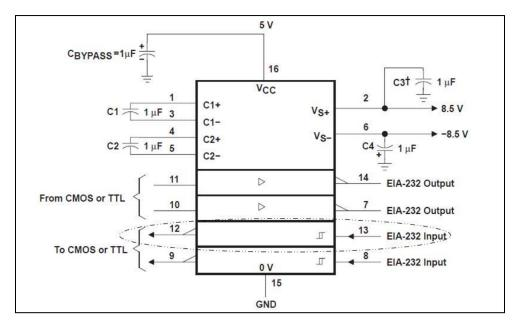
Figure 78. Max232 Port Connections
