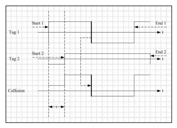
Figure 34. Superposition of Formation-0 Symbol and Formation-1 Symbol
