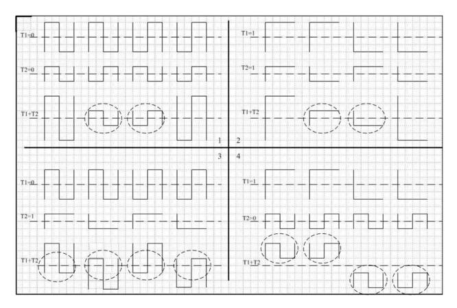
Figure 57. Collision Patterns
