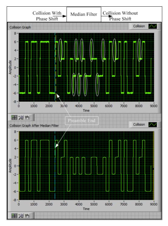
Figure 70. The Effect of Median Filter
