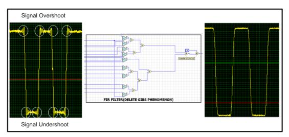
Figure 15. Signal Smoothing with 8-order FIR Filter
