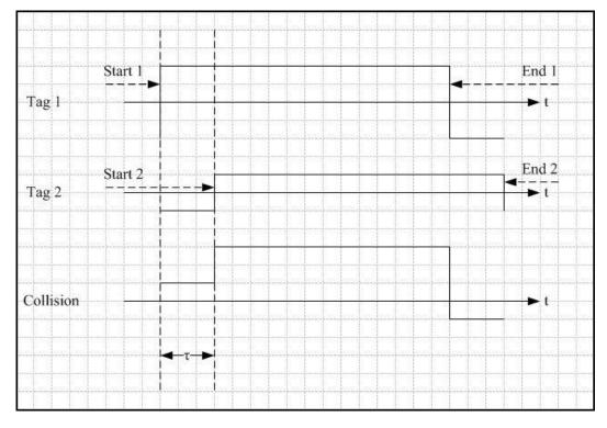
Figure 33. Superposition of Two Formation-1 Symbols
