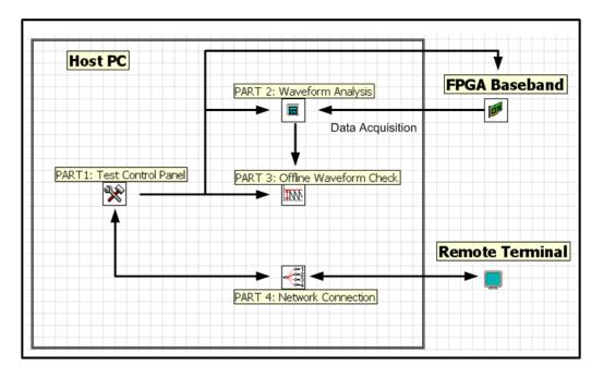
Figure 12. Platform Software Architecture
