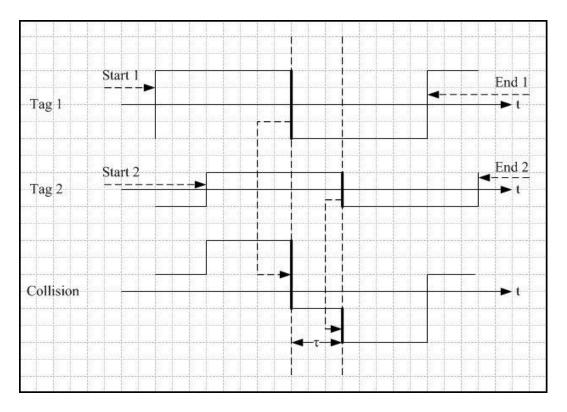
Figure 32. Superposition of Two Formation-0 Symbols
