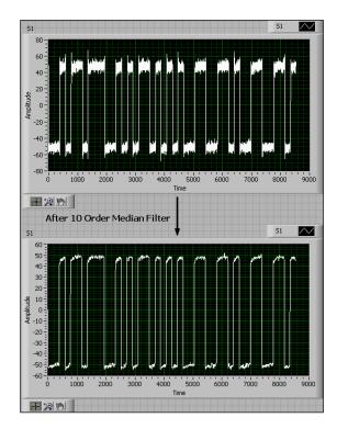
Figure 30. the effect of a 10-order median filter
