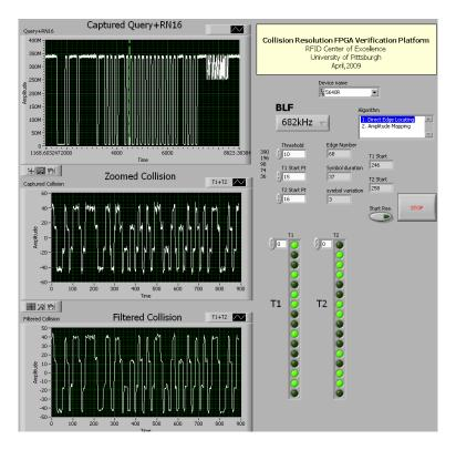
Figure 54. Resolution Result When BLF=682 kHz
