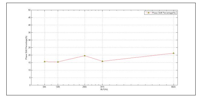
Figure 29. Tag Phase shift Percentage in Symbol duration vs. BLF (Manufacturer 2)
