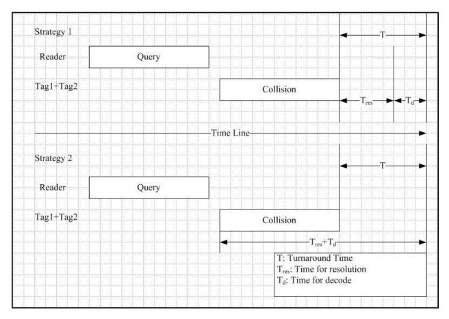
Figure 10. Collision Resolution Timing Strategy
