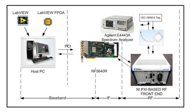
Figure 11. Platform Hardware Architecture
