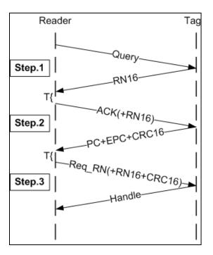
Figure 3. The Three Step Handshake
