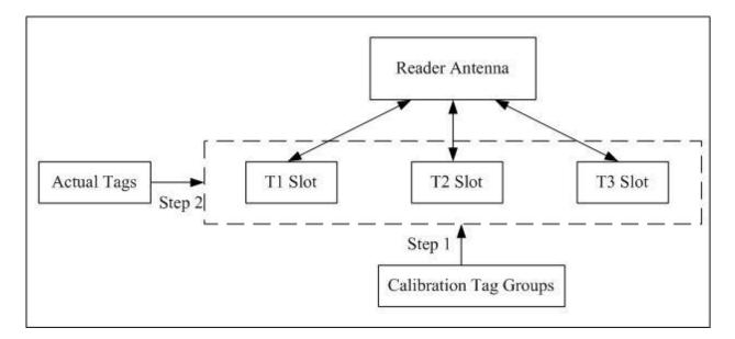
Figure 112. Calibration for Universal Whitening Matrix
