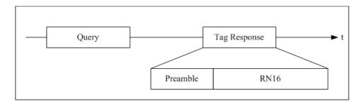
Figure 35. Tag Response Frame Architecture
