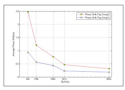
Figure 27. Tag Phase shift vs. BLF (Manufacturer 1 and Manufacturer 2)
