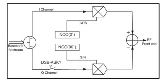
Figure 13. ASK Modulation Block
