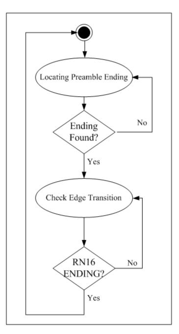
Figure 40. State Transition of the FSM
