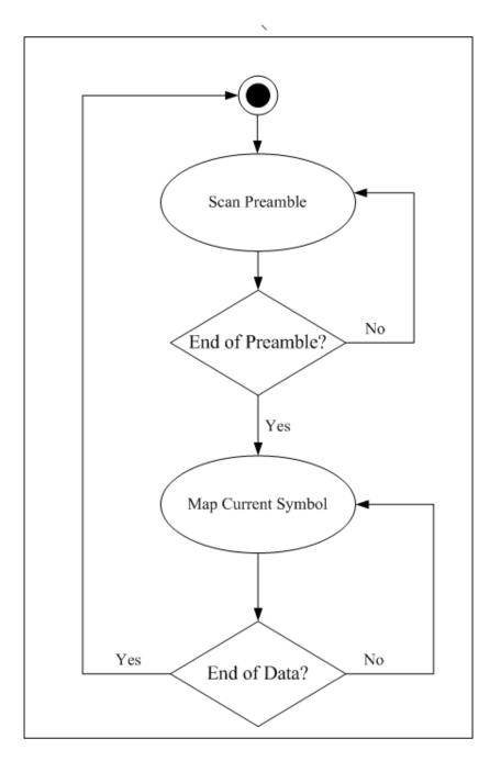
Figure 61. State Transition of FSM
