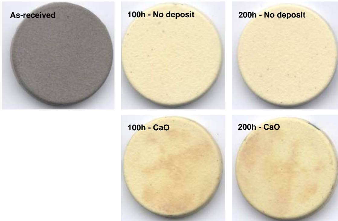
Figure 4.34 Surfaces of APS TBCs in the as-received condition and after 100 and 200 hours exposure with and without CaO deposits. The diameter of each coupon specimen is 2.54 cm.
