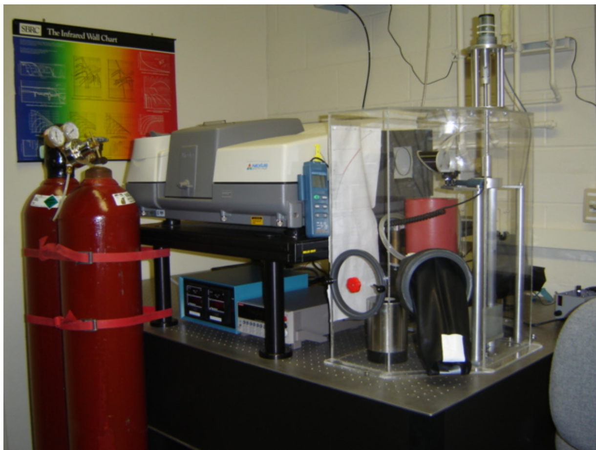
Figure 6 Photograph of the exterior of the spectrometer at the University of Pittsburgh. The main spectrometer (centre) is attached to the glovebox (right) where the samples are stored. Within the glovebox, the housing that contains the sample which is cooled by water to 25 °C (in red). Internal temperature and glovebox humidity is monitored with a hygrometer (in blue, attached to the spectrometer). The glovebox environment is purged with nitrogen (red cylinders) to reduce noise from water vapour.
