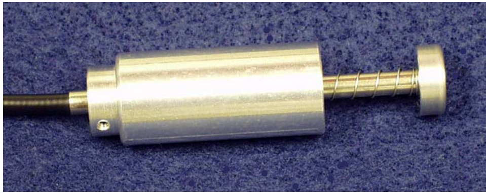
Figure 5. Fiber optic probe with indenter head and spring assembly
