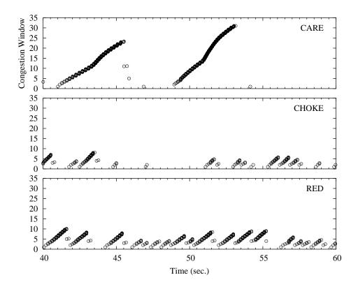
Figure 75: Congestion window behavior of TCP Reno flow number 5 under RED, CHOKe, and CARE during a time frame of 40-60 seconds.
