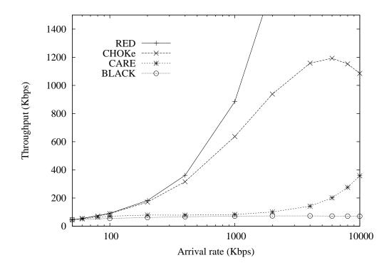
Figure 22: UDP throughput vs. arrival rate for RED, CHOKe, BLACK and CARE; Each point is an average value calculated for 20 runs.
