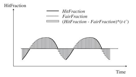
Figure 59: Simplified *HitFraction* behavior of responsive traffic under new AFC dropping policy.
