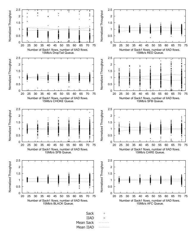
Figure 73: Normalized throughput under the scenario of Sack vs. IIAD, with drop-tail queueing, RED (first row), CHOKe, SFB (second row), SFB with tuned parameters and CARE (third row), BLACK and AFC (fourth row) where x-axis shows the equal number of flows for each type of traffic.
