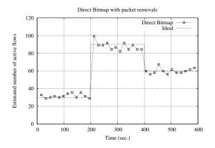
Figure 53: Estimated number of active flows Direct Bitmap with packet removals for the experiment with 30, 90, and 60 TCP flows over 600 seconds, with 250 HTTP sessions as background traffic. Max. buffer size = 300 packets.
