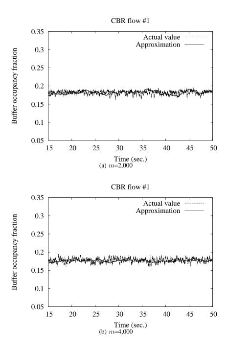
Figure 29: The effect of sample sizes (m) on approximation of the buffer occupancy fraction (continue).
