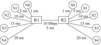
Figure 45: Ten-node dumbbell Topology with different access links' delay.
