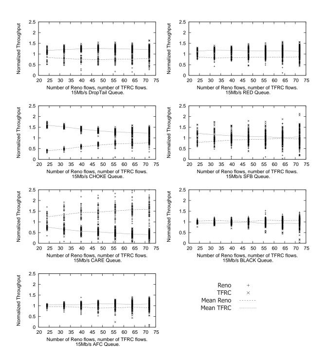
Figure 74: Normalized throughput under the scenario of Reno vs. TFRC, with drop-tail queueing, RED (first row), CHOKe, SFB (second row), CARE, BLACK (third row), and AFC (bottom) where x-axis shows the equal number of flows for each type of traffic.
