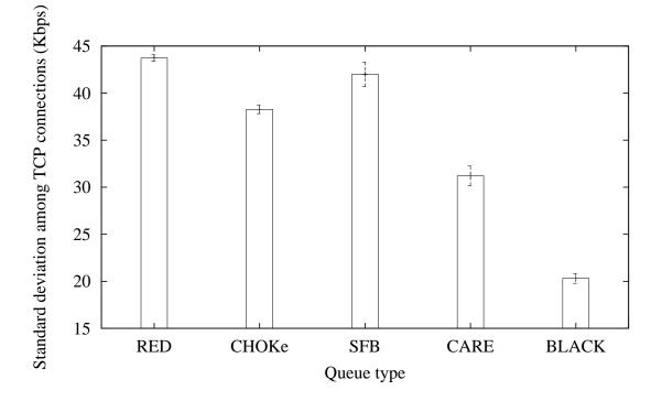
Figure 25: Standard deviation of TCP throughput under different queue types; plotted with 95% confidence interval.
