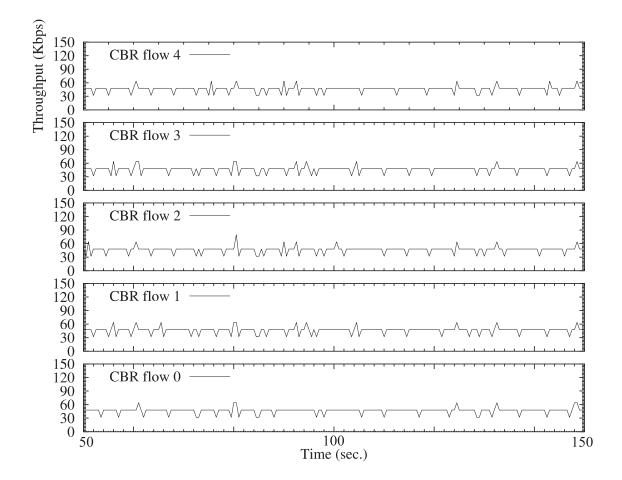
Figure 65: CBR throughput over time after passing through AFC. Bottleneck link rate is 5 Mbps and CBR arrival rate is 5 Mbps each.
