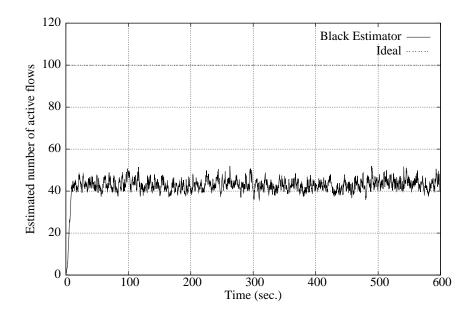
Figure 36: BLACK's estimated number of active flows for 100 TCP flows over a 45-Mbps link with 20ms delay. Maximum buffer size of 300 packets.
