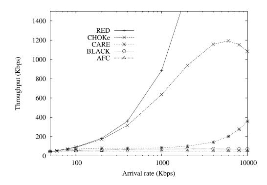
Figure 62: UDP throughput vs. arrival rate for RED, CHOKe, CARE, BLACK and AFC; Each point is an average value over 20 runs.
