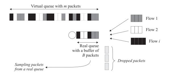
Figure 55: Virtual buffer idea to estimate a *HitFraction*.
