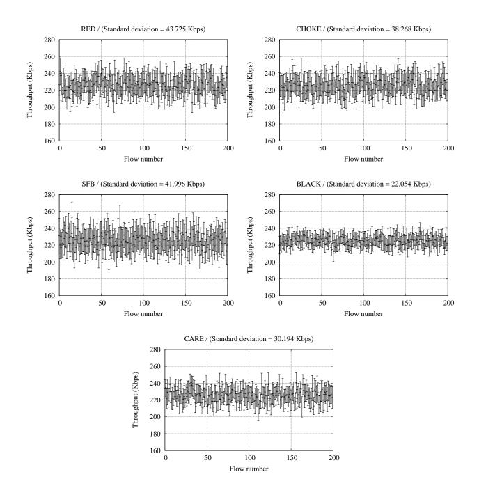
Figure 26: Per-flow TCP throughput for 200 TCP connections with different RTTs over a 45-Mbps link; plotted with 95% confidence interval.
