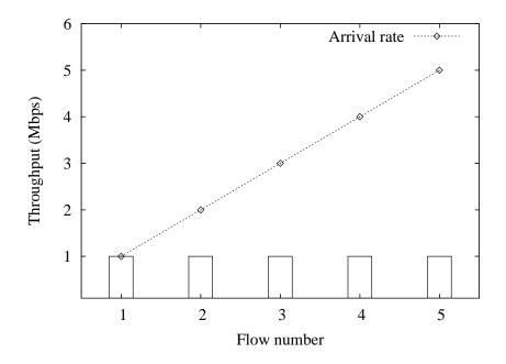
Figure 14: Simulation result showing fair throughput achieved by controlling the fair buffer occupancy fraction.
