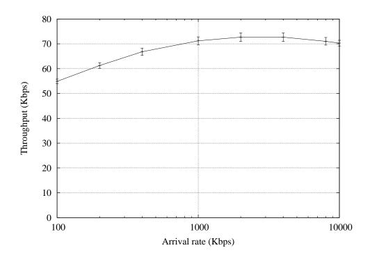
Figure 21: UDP throughput vs. arrival rate for BLACK; plotted with 95% confidence interval.
