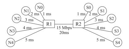
Figure 71: Simulation topology for TCP-friendly traffic experiment.
