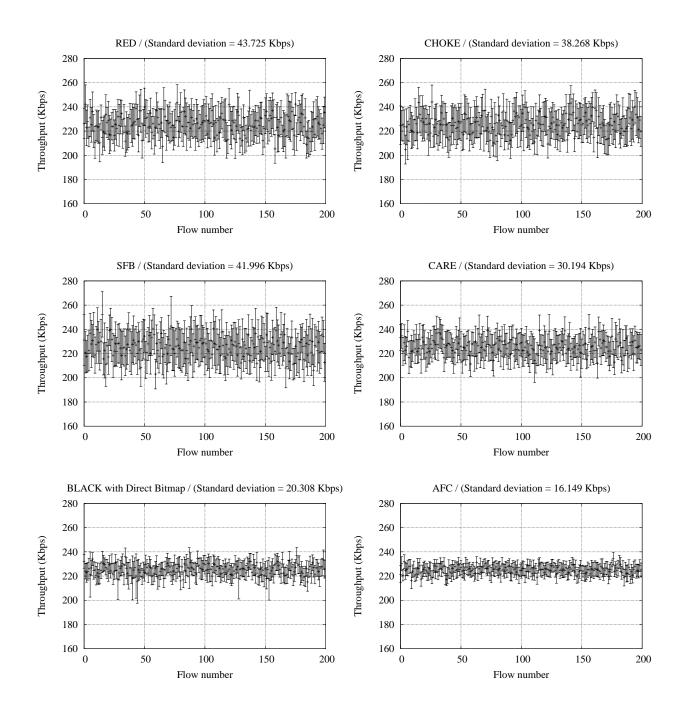
Figure 68: Per-flow TCP throughput for 200 TCP connections with different RTTs over a 45-Mbps link; plotted with 95% confidence interval. The result from AFC is included.
