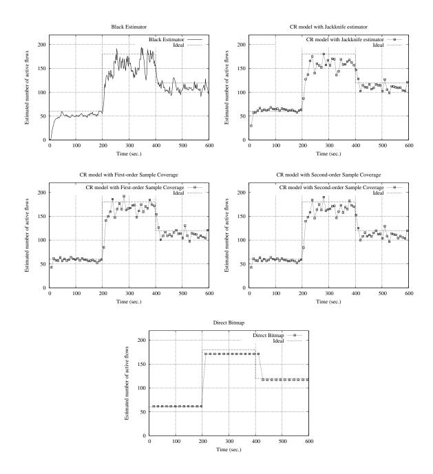
Figure 47: Estimated number of active flows for the experiment with 60, 180, and 120 TCP flows with different RTT over 600 seconds.
