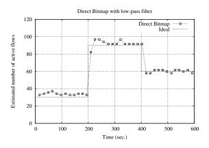
Figure 52: Estimated number of active flows using Direct Bitmap with low-pass filter for the experiment with 30, 90, and 60 TCP flows over 600 seconds, with 250 HTTP sessions as background traffic.
