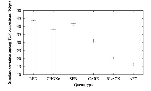
Figure 67: Standard deviation of TCP throughput under different queue types; plotted with 95% confidence interval.
