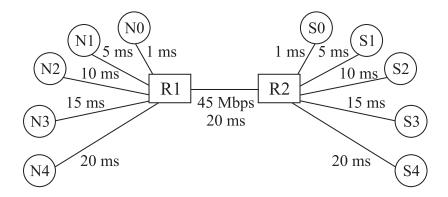
Figure 24: Simulation topology for TCP with different round-trip times.
