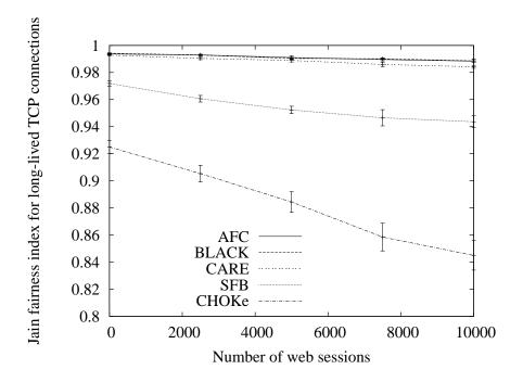
Figure 70: Jain's fairness index among long-lived TCP connections at different background web traffic loads. The legend represents the lines in the figure from top to bottom respectively.
