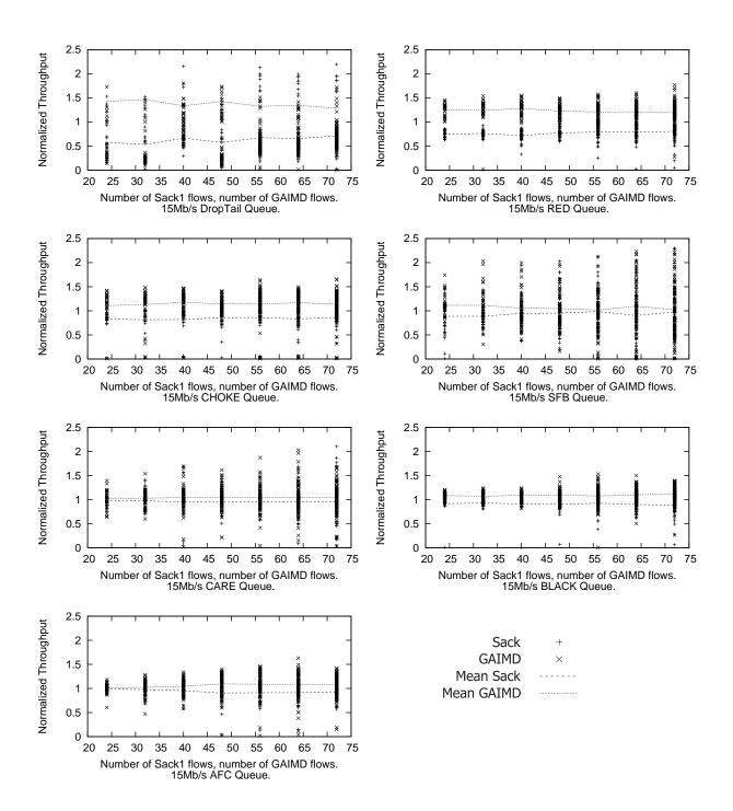
Figure 72: Normalized throughput under the scenario of Sack vs. GAIMD(1,1/8), with drop-tail queueing, RED (first row), CHOKe, SFB (second row), CARE, BLACK (third row), and AFC (bottom) where x-axis shows the equal number of flows for each type of traffic.
