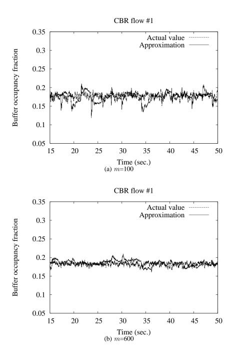
Figure 28: The effect of sample sizes (m) on approximation of the buffer occupancy fraction.
