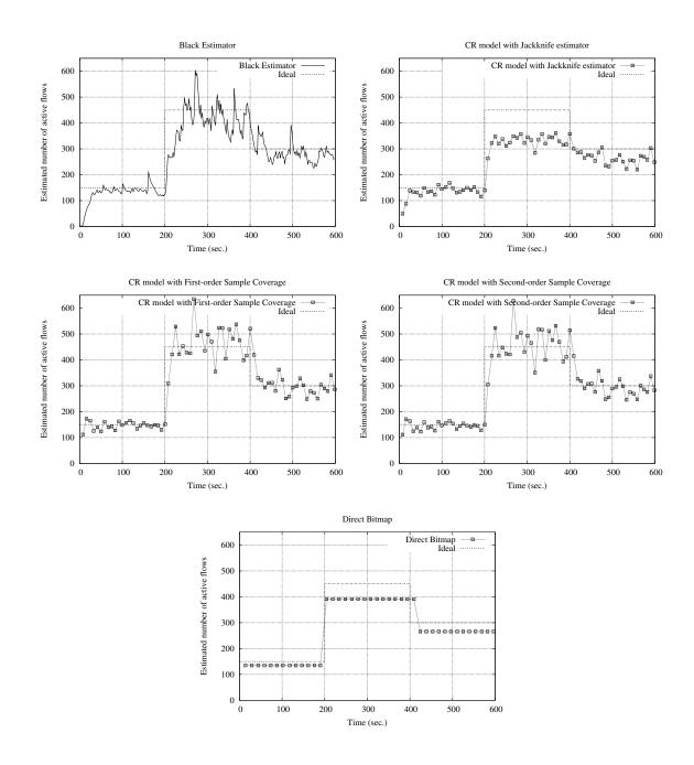
Figure 44: Estimated number of active flows for the experiment with 150, 450, and 300 TCP flows over 600 seconds.
