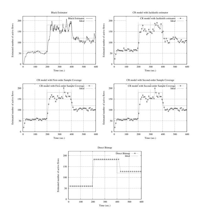
Figure 43: Estimated number of active flows for the experiment with 60, 180, and 120 TCP flows over 600 seconds.
