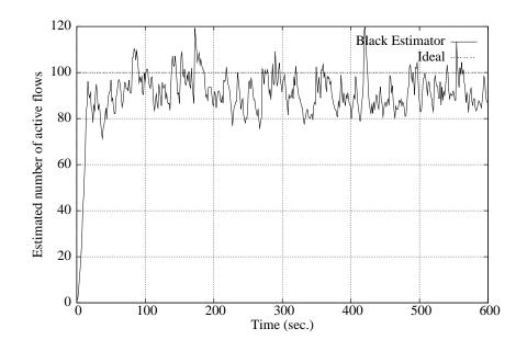
Figure 35: BLACK's estimated number of active flows for 100 TCP flows over a 10-Mbps link with 5ms delay. Maximum buffer size of 300 packets.
