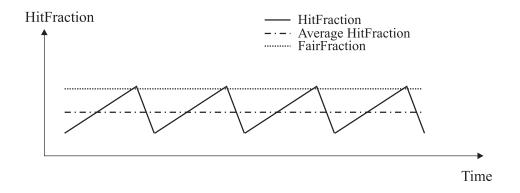
Figure 58: Simplified *HitFraction* behavior of responsive traffic under AFC dropping policy with no credit-based mechanism.
