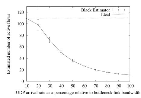
Figure 40: BLACK's estimated number of active flows for 100 TCP flows and 10 UDP flow over a 10-Mbps link with 20ms delay. UDP arrival rate varies from 10% to 100% of bottleneck link bandwidth.
