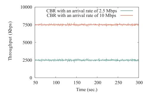
Figure 79: Simulation result of the parallel parking lot scenario; showing the throughput obtained by the flow from node 1 to node 2 (10 Mbps) and the flow from node 1 to node 5 (2.5 Mbps).
