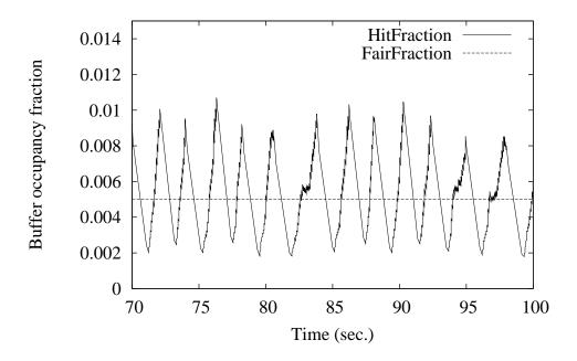
Figure 60: Evolution of *HitFraction* over time of a sample flow under AFC with a credit-based mechanism.
