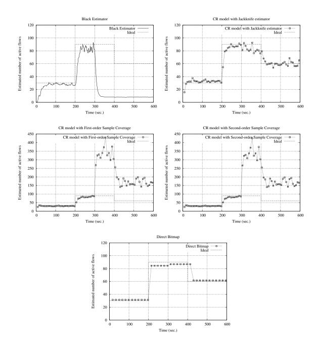
Figure 49: Estimated number of active flows for the experiment with 30, 90, and 60 TCP flows over 600 seconds, with UDP traffic consuming 33% of bottleneck link bandwidth starting at 300 seconds.
