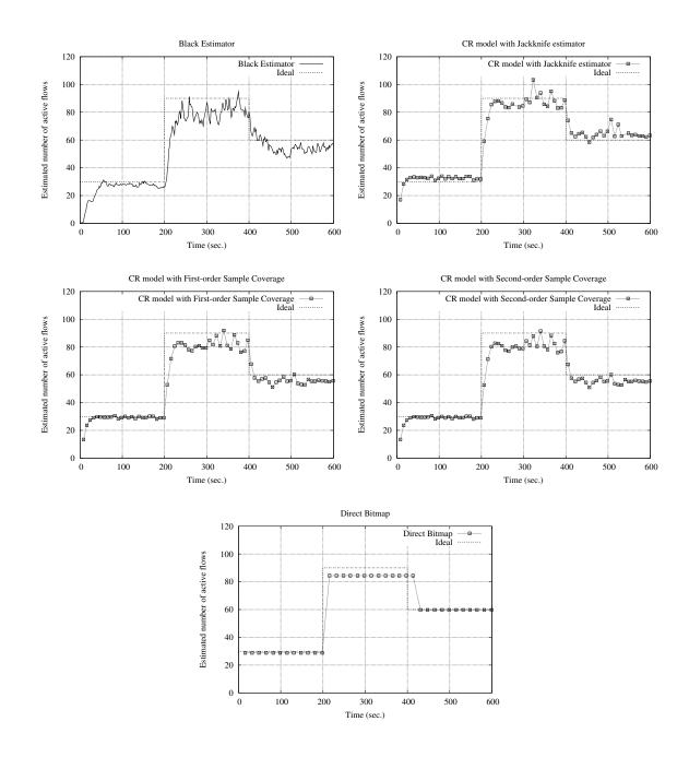
Figure 42: Estimated number of active flows for the experiment with 30, 90, and 60 TCP flows over 600 seconds.
