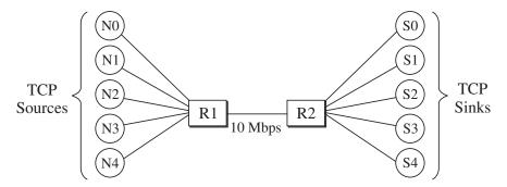
Figure 18: Simulation topology for pilot experiment on the estimation of the number of active flows.
