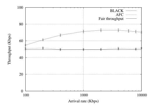
Figure 61: UDP throughput vs. arrival rate for BLACK and AFC; plotted with 95% confidence interval.
