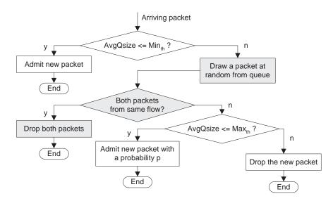
Figure 10: The CHOKe algorithm [52].
