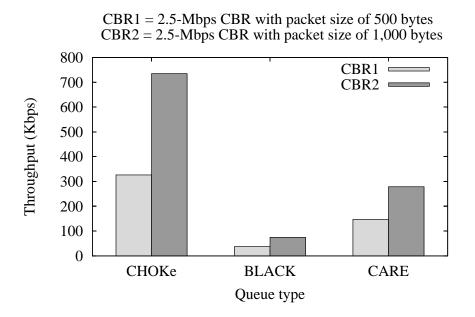
Figure 32: Average throughput of two CBR traffic flows with packet sizes of 500 bytes and 1,000 bytes, under CHOKe, BLACK, and CARE.
