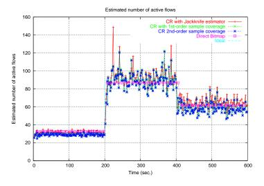
Figure 41: Estimated number of active flows for the experiment with 30, 90, and 60 flows over 600 seconds.
