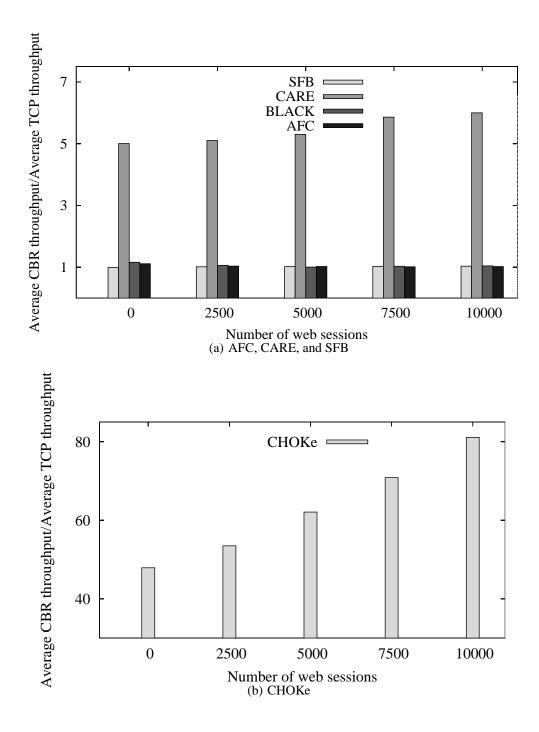
Figure 69: Average per-flow CBR throughput over average per-flow TCP throughput (average over 20 runs) at different background web traffic loads.
