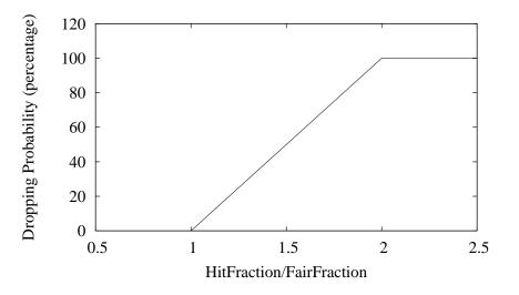
Figure 57: Dropping probability as a function of *HitFraction/FairFraction* of BLACK.
