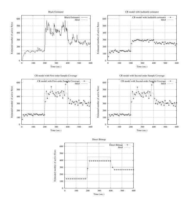
Figure 48: Estimated number of active flows for the experiment with 150, 450, and 300 TCP flows with different RTT over 600 seconds.
