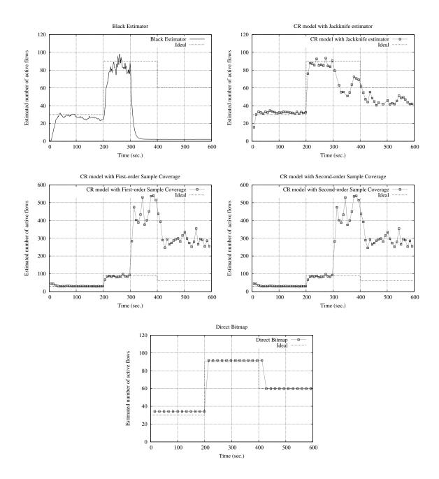
Figure 50: Estimated number of active flows for the experiment with 30, 90, and 60 TCP flows over 600 seconds, with UDP traffic consuming 66% of bottleneck link bandwidth starting at 300 seconds.
