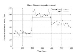
Figure 54: Estimated number of active flows Direct Bitmap with packet removals for the experiment with 30, 90, and 60 TCP flows over 600 seconds, with 250 HTTP sessions as background traffic. Max. buffer size = 1000 packets.
