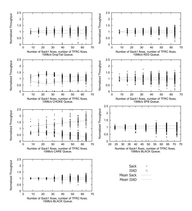
Figure 77: Normalized throughput under the scenario of Sack vs. TFRC, with drop-tail queueing, RED (first row), CHOKe, SFB (second row), SFB with tuned parameters and CARE (third row), BLACK and AFC (fourth row) where x-axis shows the equal number of flows for each type of traffic.
