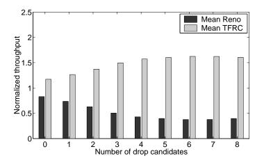
Figure 76: Comparing average normalized throughput of 40 TCP Reno traffic and 40 TFRC traffic under CHOKe with different number of drop candidates.
