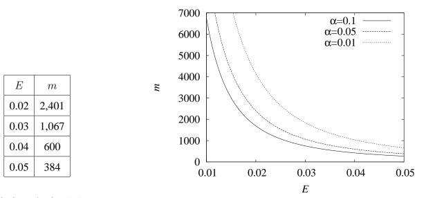
Table 8: Sample size (m) as afunction of E with 95% con-fidence. $100(1 - \alpha)$  confidence.
