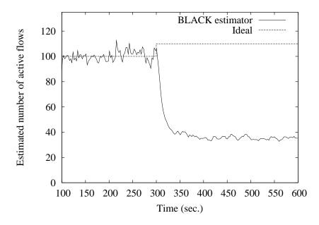
Figure 39: BLACK's estimated number of active flows for 100 TCP flows and 10 UDP flow over a 10-Mbps link with 20ms delay. UDP traffic start at 300 seconds and consume half of the bottleneck link bandwidth.
