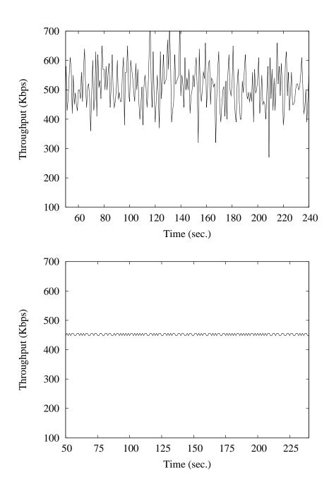
Figure 64: CBR throughput over time after passing through BLACK and AFC. Bottleneck link rate is 45 Mbps and CBR arrival rate is 10 Mbps.
