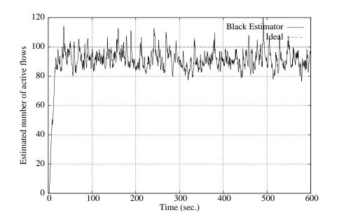
Figure 37: BLACK's estimated number of active flows for 100 TCP flows over a 45-Mbps link with 20ms delay. Maximum buffer size of 3,000 packets.
