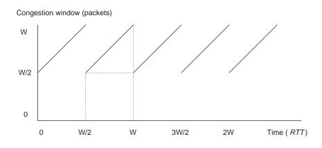
Figure 6: TCP congestion window behavior in steady state of a simplified model.
