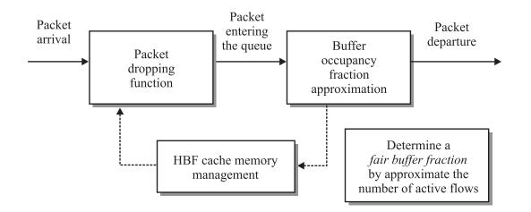
Figure 56: AFC components and a flow of packets that pass through the queue (shown in a solid arrow line).
