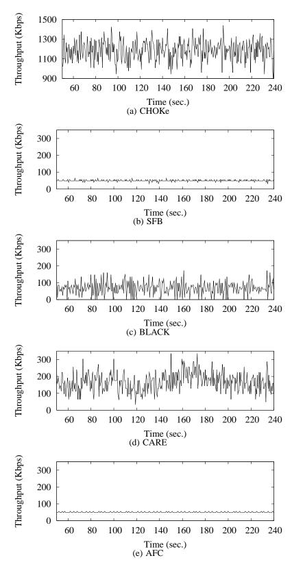
Figure 63: CBR throughput over time after passing through different fair AQM schemes. Bottleneck link rate is 5 Mbps and CBR arrival rate is 5 Mbps.
