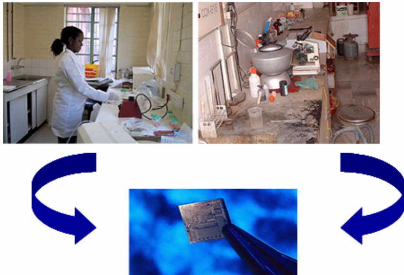
Figure 1.1 Illustration of the goal of lab-on-a-chip microsystems, to integrate multiple laboratory functions onto a single chip [44],[45].
