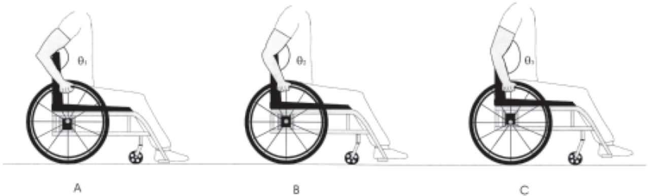
Figure 1: Difference in elbow flexion angle (Q). Diagram A = Angle is too small, Diagram B = Correct angle (100-120 deg.), Diagram C = Angle is too large. (Source: PVA CPG—Preservation of Upper Limb Function Following Spinal Cord Injury)
