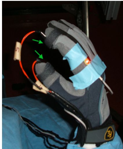
Figure 3.6: Vibrotactile feedback system (VIPER). Tactors are positioned on the fingertips of the thumb and index finger (green arrows) to apply continuous, graded vibrotactile feedback. Also shown is an active marker (red LED) attached to the back of the index finger, which is used by the motion capture system to track hand position.
