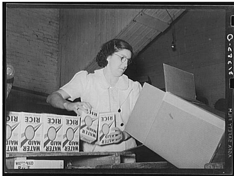
Figure 15: Russell, L. (1938c). Removing packages of rice from conveyer to place them in fiber cartons. State rice mill, Abbeville, Louisiana. (Library of Congress, Prints & Photographs Division, FSA/OWI Collection, [LC-USF34-031383-D (b&w film neg.)]
