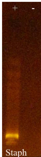
Figure 34: Using electrophoresis for detection of same solution from Figure 32. The left hand lane shows DNA extraction indicating an infection. The right hand side shows no DNA extraction. This image is taken when the products have been electrophoresed and are excited with UV light.
