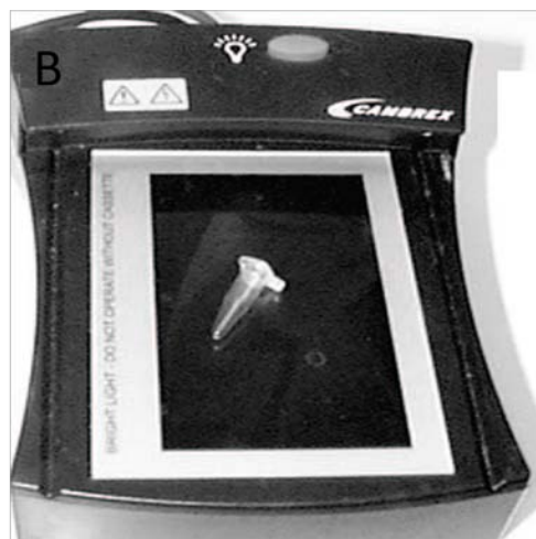
Figure 4: A UV transilluminator is shown with a test tube on top. The UV transilluminator is not portable. Taken from reference 2.
