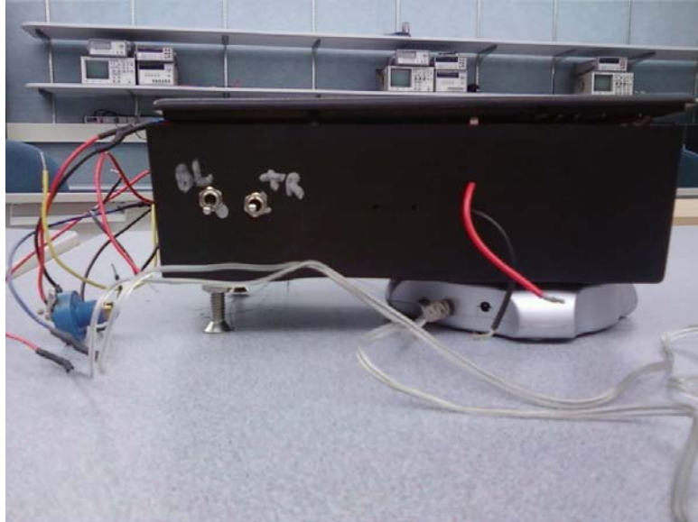
Figure 27: LAMP box sitting on top of USB heater. Screws used for balancing on left hand side.
