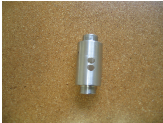
Figure 4.4 photograph of the magnet sleeve with increased magnetic field length
