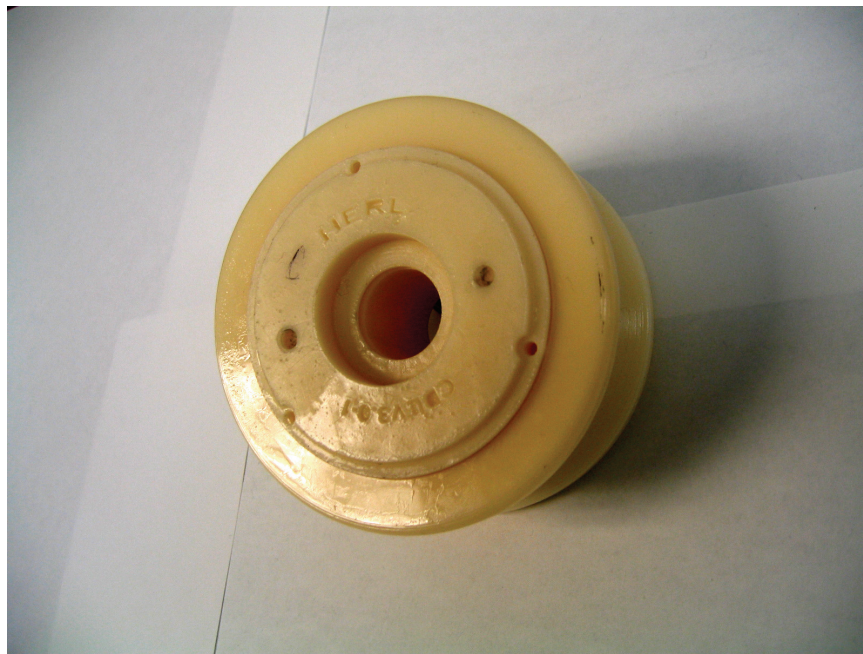
Figure 5.3 Photograph the CDL 3.0 concept fabricated using SLA
