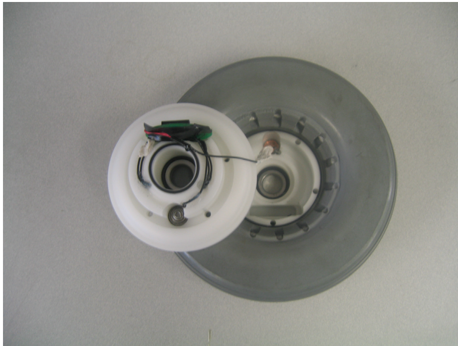
Figure 3.7 Photograph two halves of the CDL v2.2 hub with inside exposed.
