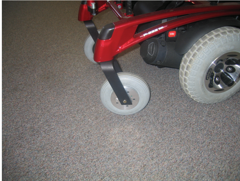
Figure 3.10 Photograph of the aluminum CDL v2.0 installed on a rear wheel drive EPW.
