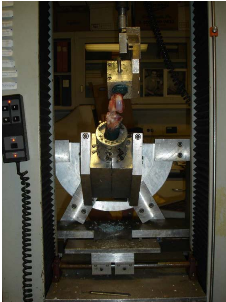
Figure 10. Femur-ACL-tibia complex mounted within custom clamps on a materials testing machine for uniaxial tensile testing.
