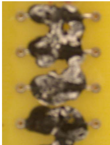
Figure 30: Salt formation on the PEDOT samples from unused \text{Na}_2\text{S}_2\text{O}_8 .
