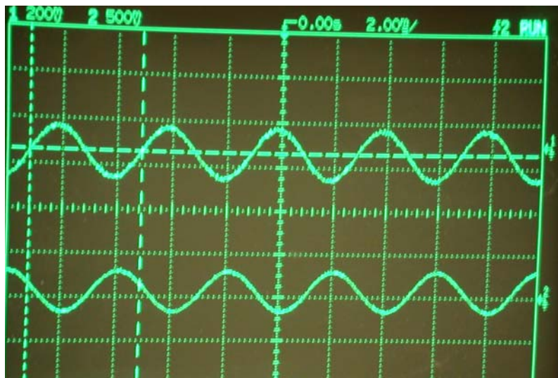
Figure 18: Rectification test results of sample number 10 at 30 MHz.
