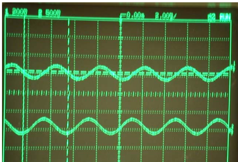
Figure 29: Rectification test results of sample number 5 at 30 MHz.
