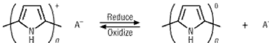
Figure 45: The oxidation reduction reaction of a conjugated polymer.
