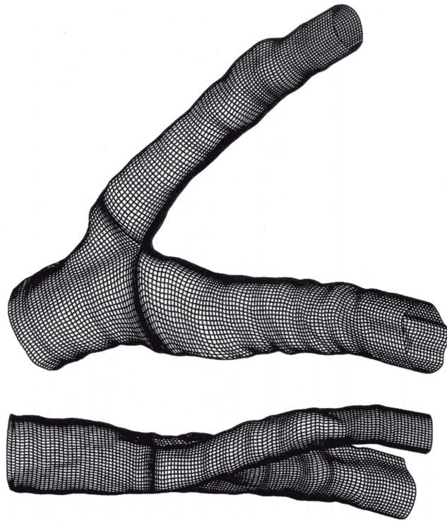
Figure 1.10 Figure from [94] showing the CFD model of the reconstructed left anterior descending coronary artery bifurcation.
