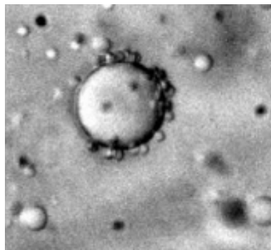
Figure 23. OTS-silica particles adsorb on surface of a PEO drop in PIB.
