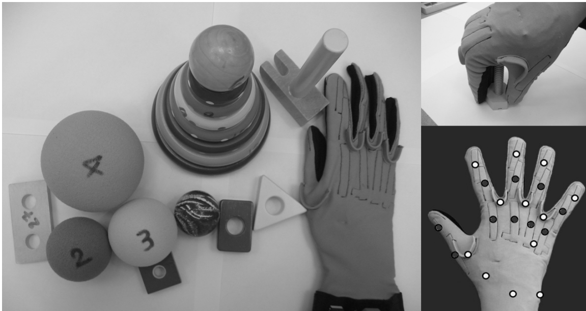
Figure 10. CyberGlove with grasping objects, sensors used (dark) and custom grasp
