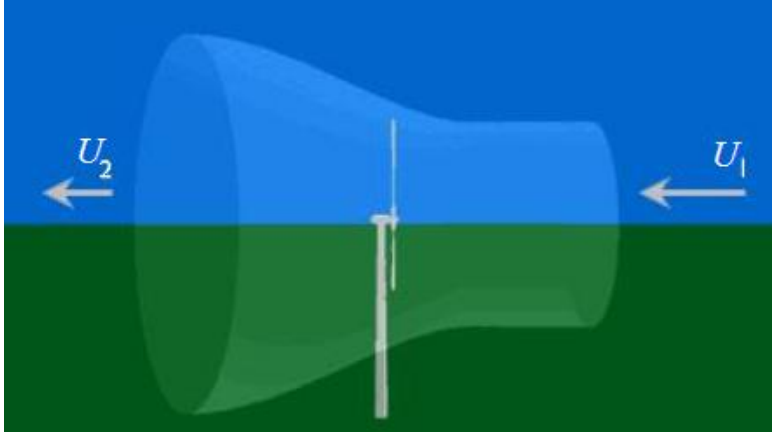
Figure 2: Betz law control volume; an imaginary stream tube, which shows how the slow moving wind behind a turbine must occupy a larger volume than the faster moving wind before the turbine [3]
