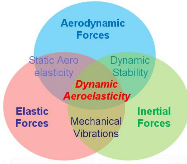
Figure 17: Aeroelastic Triangle; significant interaction among the triangle's forces results in multimode flutter
