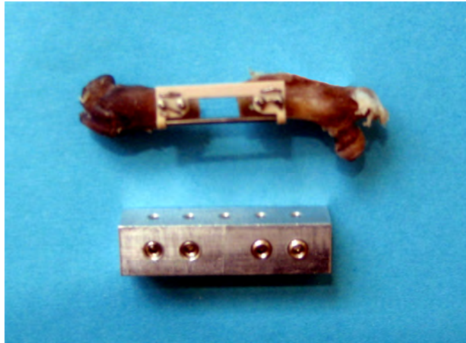
Figure 2.10. Novel fixator in place across a rat, femoral 5mm defect. The stability bar of first generation, ExFixOld, is shown below for comparison.
