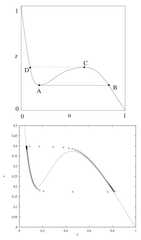
Figure 1.3. Plot of 0 = -u + (1 - z)f(u) with points relevant to the relaxation oscillation labeled. Below is a numerically computed solution with r = 300 illustrating the relaxation character of the oscillation.
