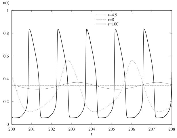
Figure 1.1. The behavior of (1.1) for different values of the parameter  $r = R/\tau$  with  $f(u) = 1/(1 + \exp(-8(u - .333)))$ . The period of the smallest oscillation is 4 and that of the largest is 1.43.
