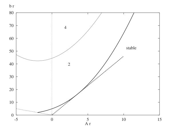
Figure 1.2. Stability diagram for (1.4) as a function of Ar and br. Straight lines depicts the curve b = -A and b = A/M where M is defined in the text. The remaining curves depict lines along which there are purely imaginary roots. Numbers denote the number of eigenvalues with positive real parts.
