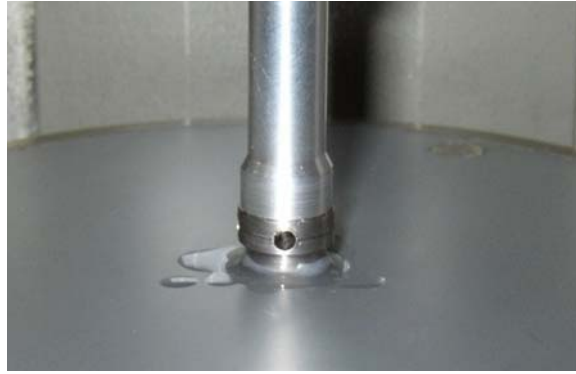
Figure 4.5 Photograph showing fixtured NP with mineral oil applied.
