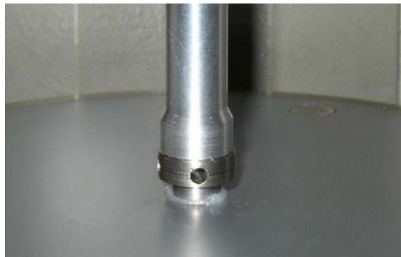
Figure 4.4 Photograph of fixtured NP specimen. Geometry gap is completely filled.
