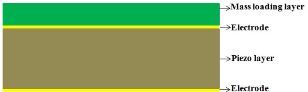
Figure 5.8. The schematic of FBAR for mass sensor application
