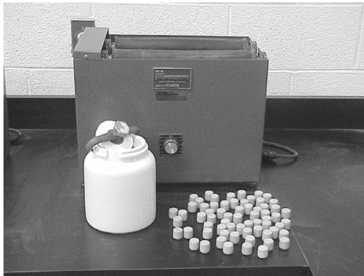
Figure 39 Jar Milling Apparatus Including the Jar and the Lid, the Charges and the Roller Milling Machine
