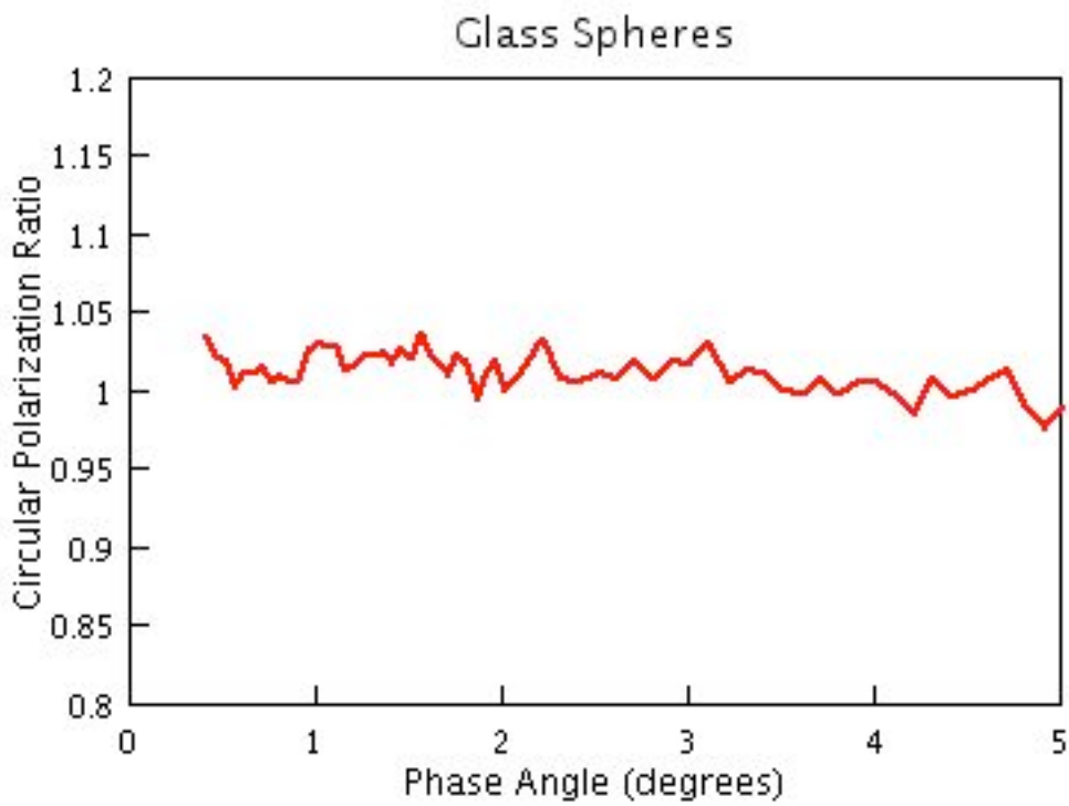
Figure 20b: Phase curve and circular polarization ratio data for 2.5 μm glass microspheres
