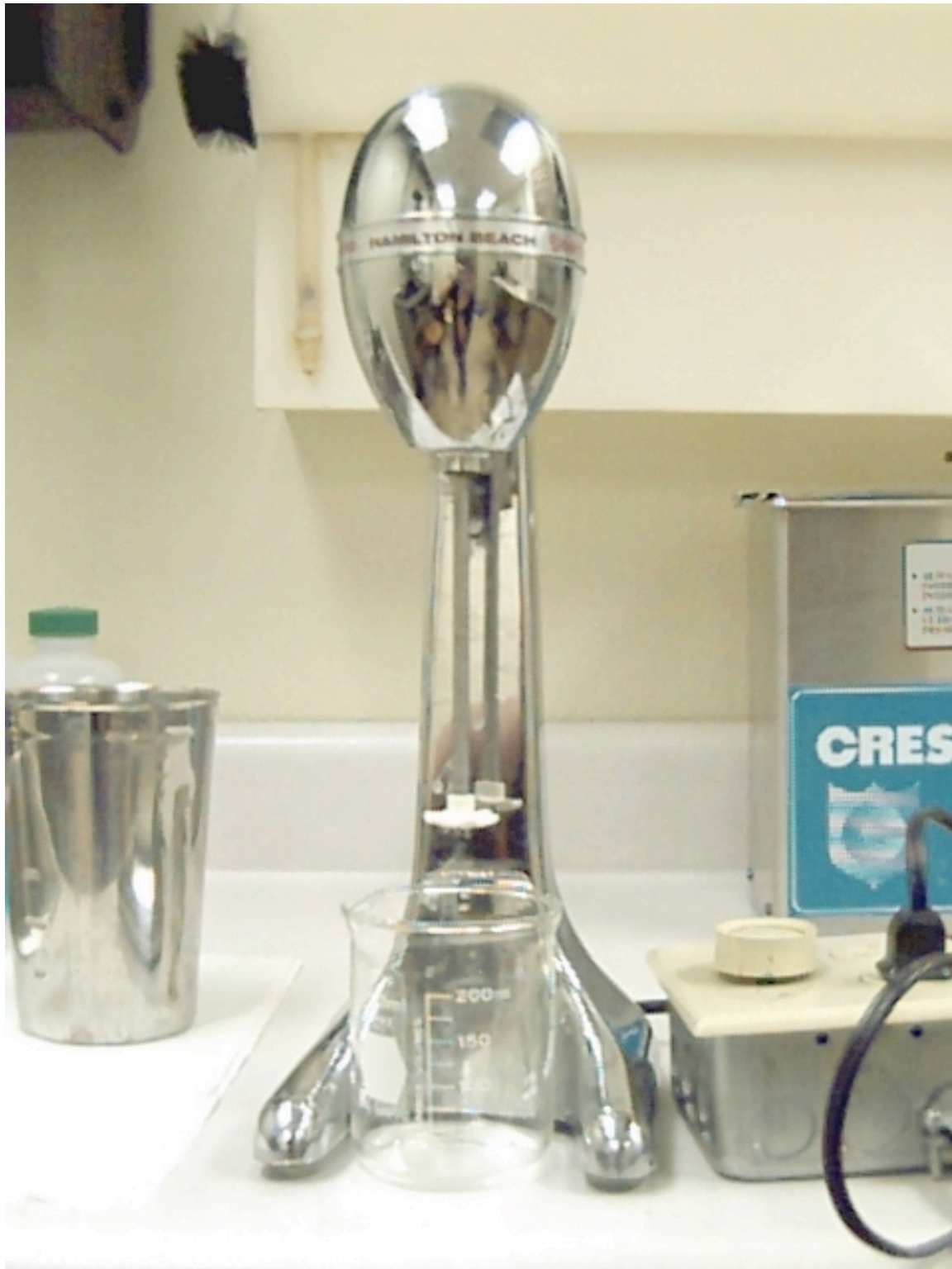
Figure 4: Image of shear stress generator used during CCSEM sample preparation (e.g. Hamilton Beach Mixmaster milkshake machine).
