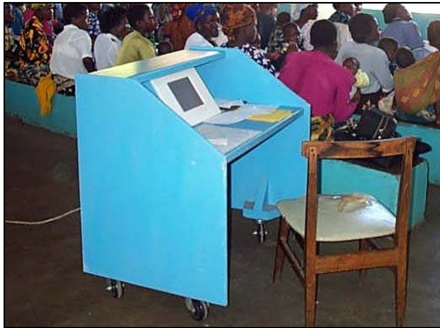
Figure 5: Plywood desk containing workstation, printer, battery and charger
