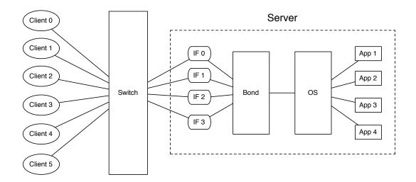
Figure 4: Basic experimental setup
