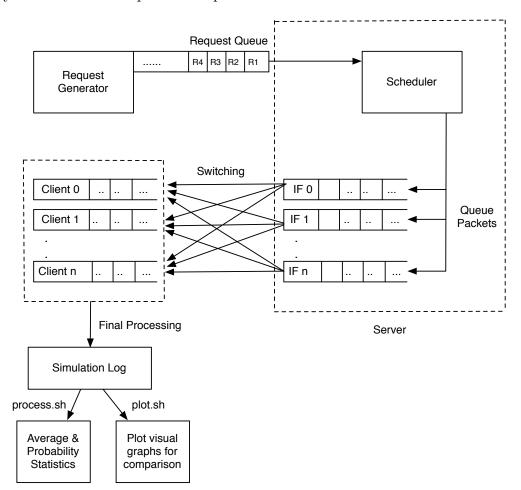
Figure 5: Bonding Simulator Design
