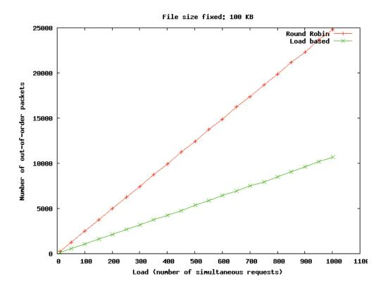
Figure 9: Impact of load on with fixed file size - 100KB
