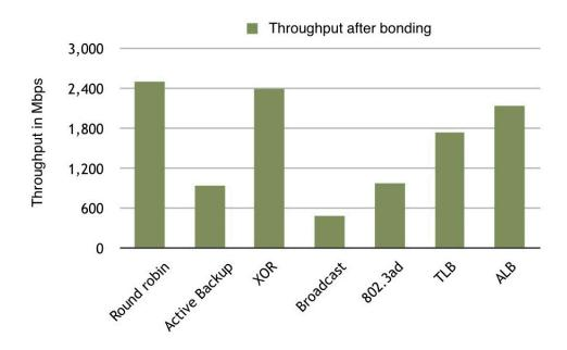
Figure 3: Throughput with different modes
